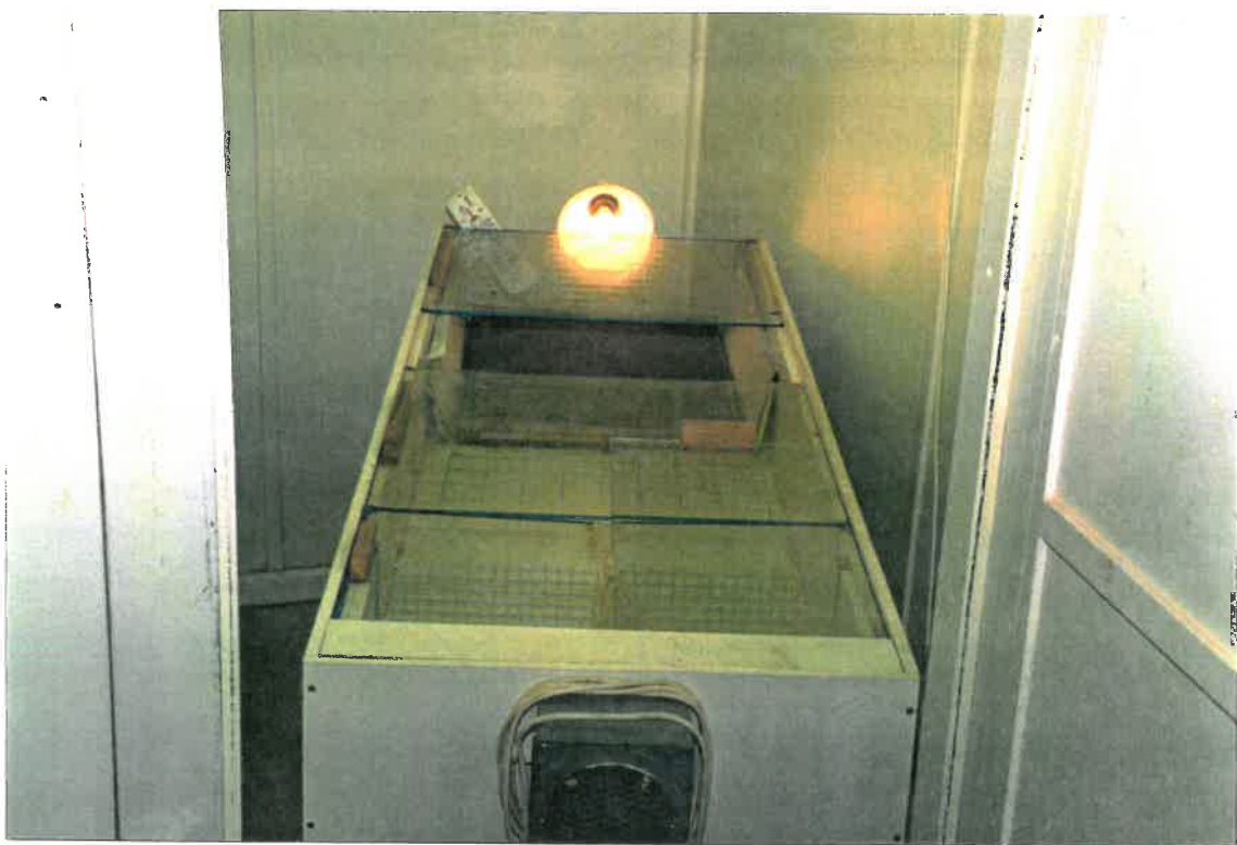
Fig 3.2 A photograph showing the wind tunnel used in this experiment.
