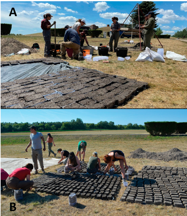
Figure 8. Project members A) screening and saturating soil with water and B) removing bricks from formers to cure in the sun.
