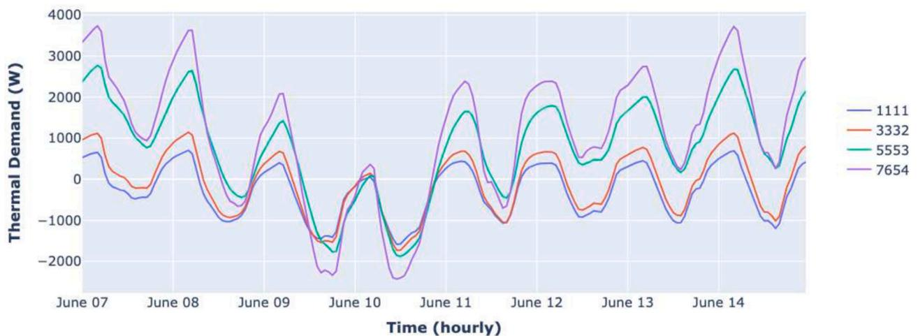
Fig. 15. Effects of thermal efficiency on the hourly cooling demand for a detached house in Cardiff oriented at 0° (north-facing).
