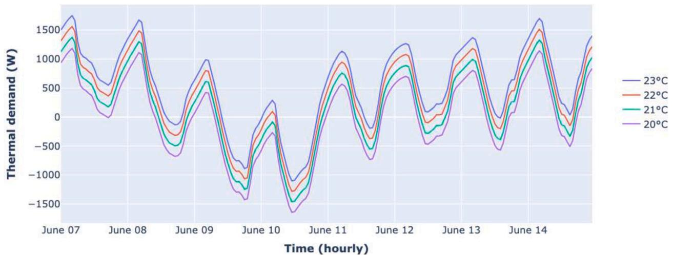
Fig. 5. Comparison of hourly thermal demand with different thermostat temperatures for a typical design year. Detached house in Cardiff at orientation 0° (i.e. north-facing) with a building code '3244'.
