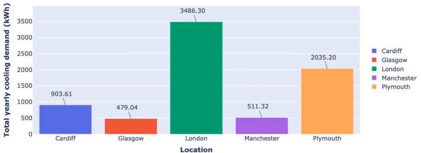
Fig. 19. Total yearly cooling demand for a north-facing (orientation of  $0^\circ$ ), lowly thermally efficient (building code '7654') detached house at different locations in the UK.
