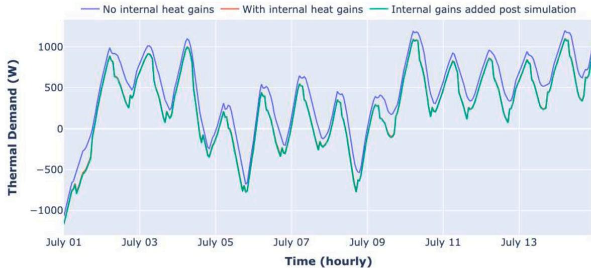
Fig. 22. Effect of internal heat gains in the cooling demand of a ground floor flat in Cardiff with the lowest thermal efficiency (building code '7654') and orientation of  $0^\circ$ .
