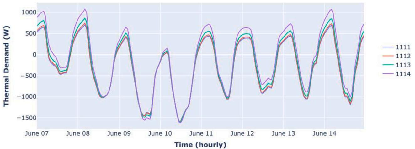
Fig. 16. Effects of window construction on the hourly cooling demand for a detached house in Cardiff oriented at 0° (north-facing).
