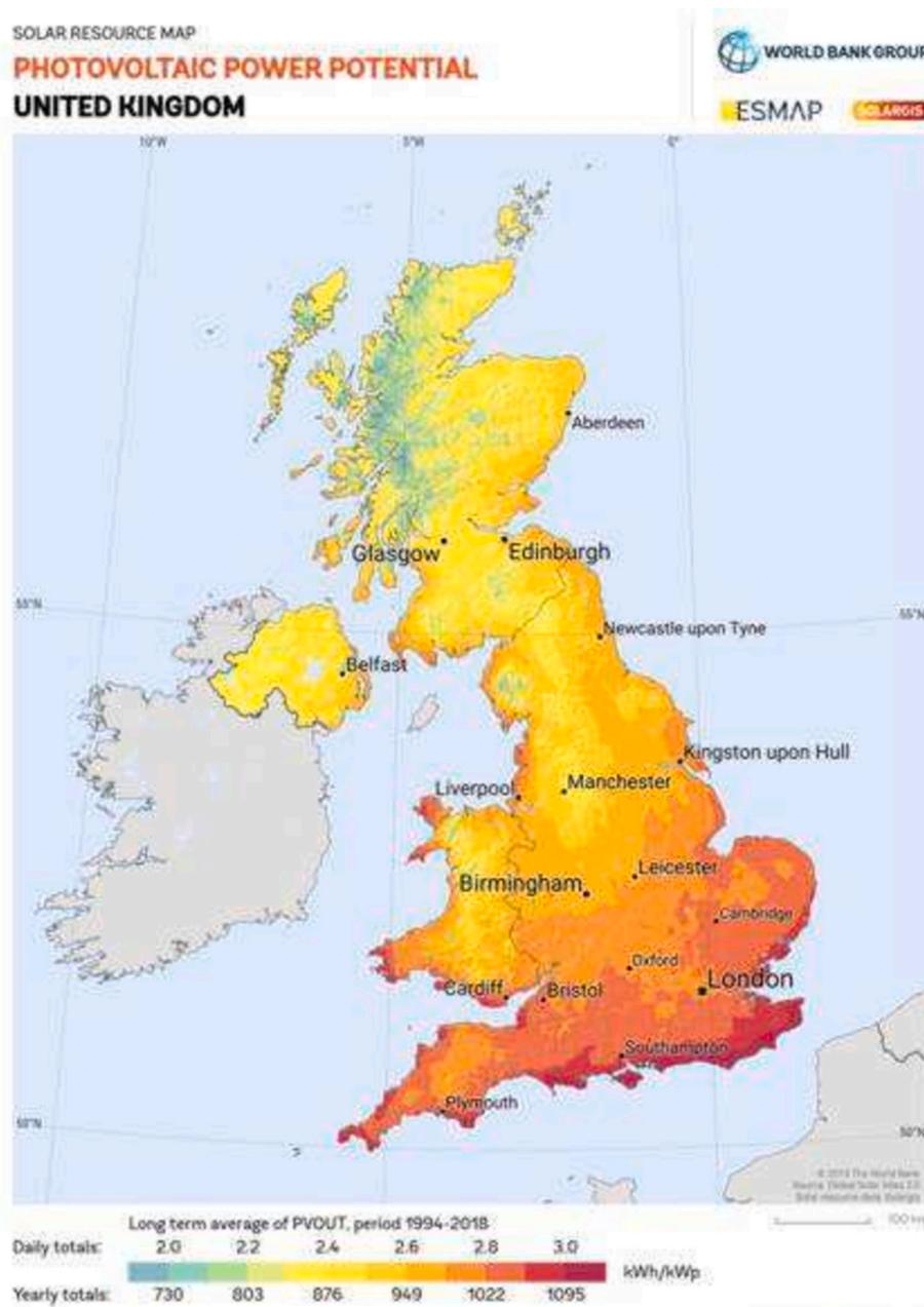
Fig. 4. Photovoltaic power potential in the UK [44].
