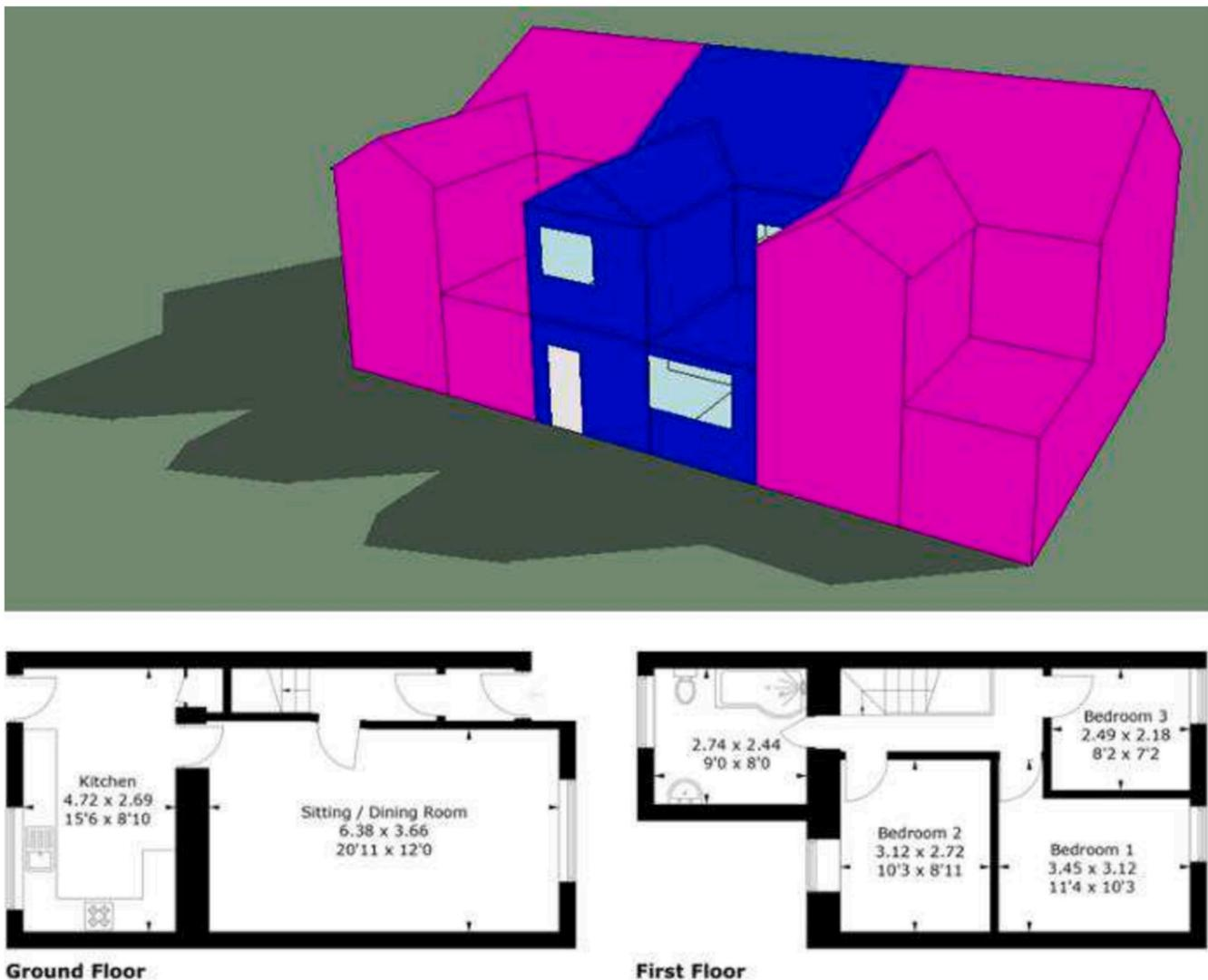
**Fig. 2.** Three-dimensional model of a terraced house produced in IES VE using a layout obtained from [27]. The blue shading represents the dwelling under investigation and the pink shading the adjacent buildings. (For interpretation of the references to colour in this figure legend, the reader is referred to the web version of this article.)
