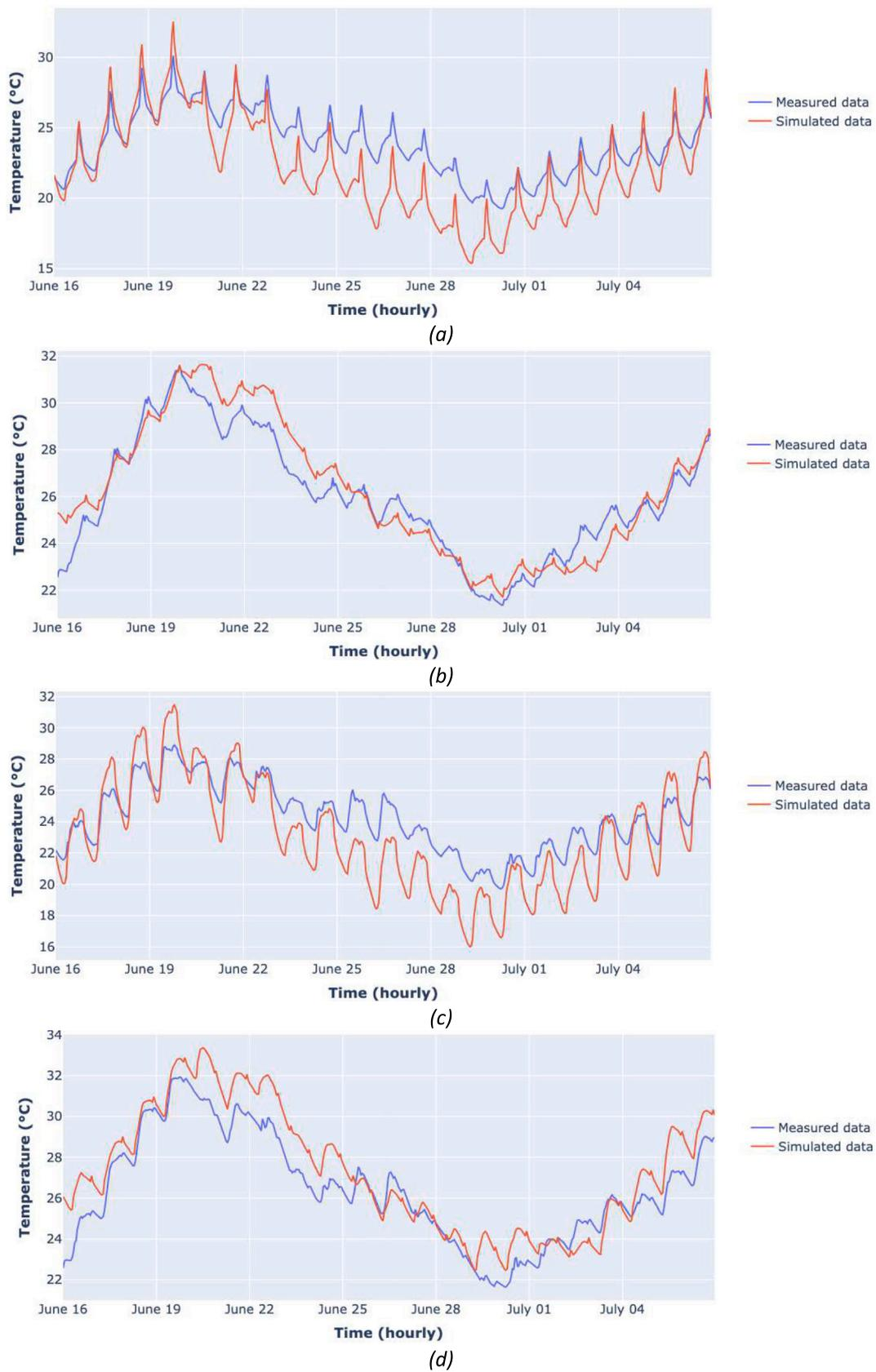
Fig. 9. Comparison of internal room temperatures using IES VE with measured values reported in [16]: (a) kitchen; (b) rear bedroom; (c) living room; (d) front bedroom.
