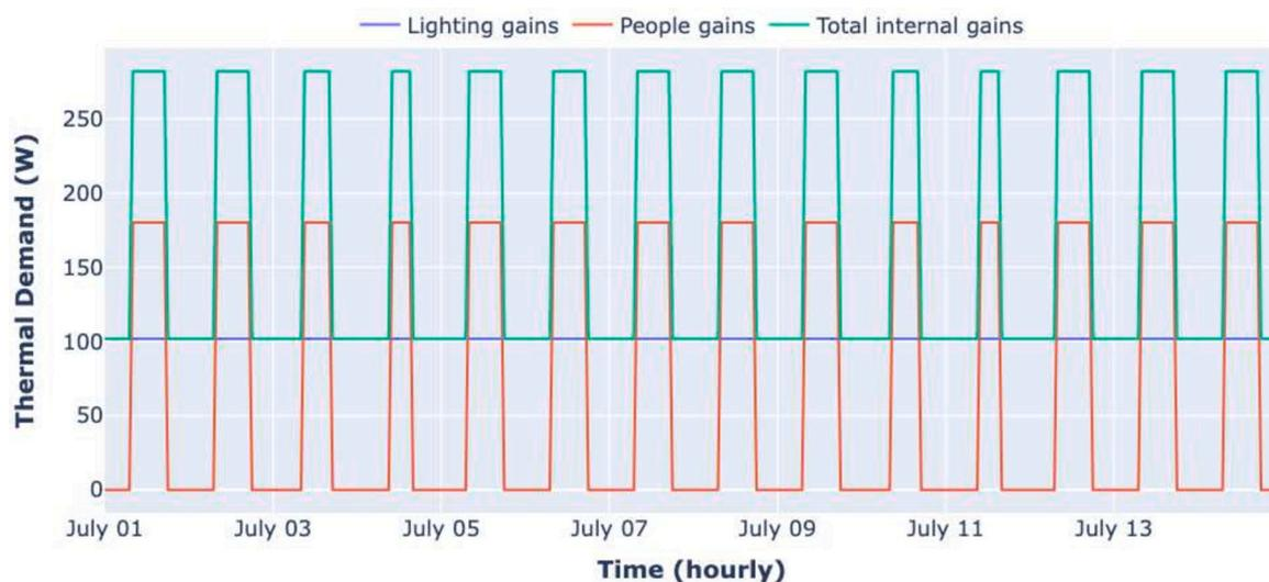
Fig. 20. Internal heat gains for a ground floor flat.
