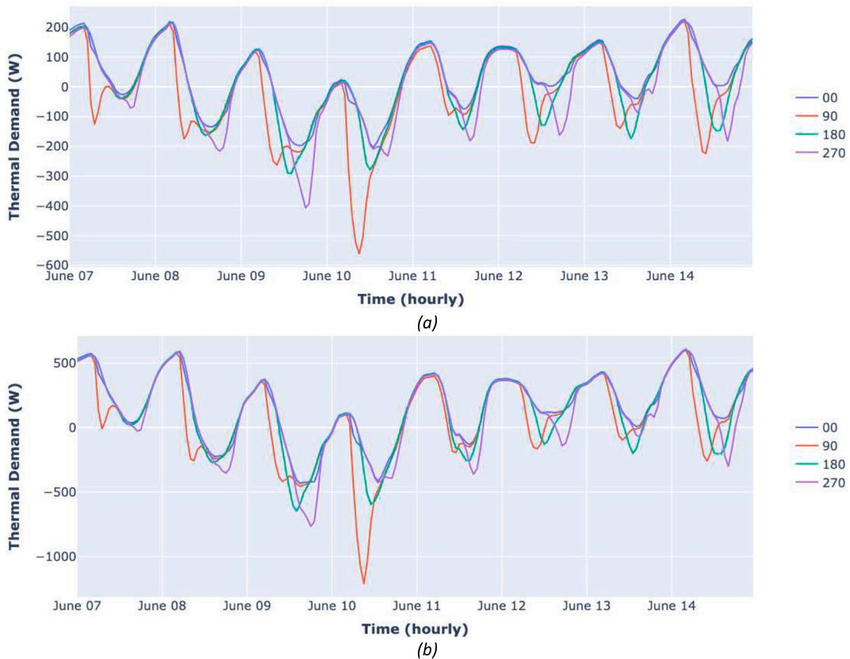
Fig. 14. Effects of external wall orientation on the hourly cooling demand for a middle-floor flat in Cardiff. Flat with the (a) highest thermal efficiency (building code '1111'), (b) lowest thermal efficiency (building code '7654').
