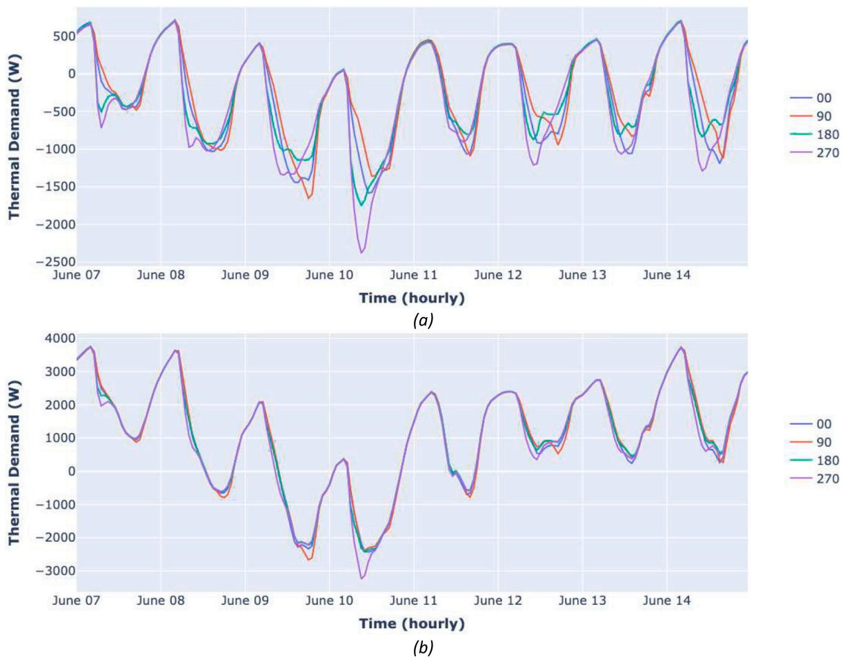
Fig. 17. Effects of orientation on the hourly cooling demand for a detached house in Cardiff. Dwelling with the (a) highest thermal efficiency (building code '1111'); (b) lowest thermal efficiency (building code '7654').
