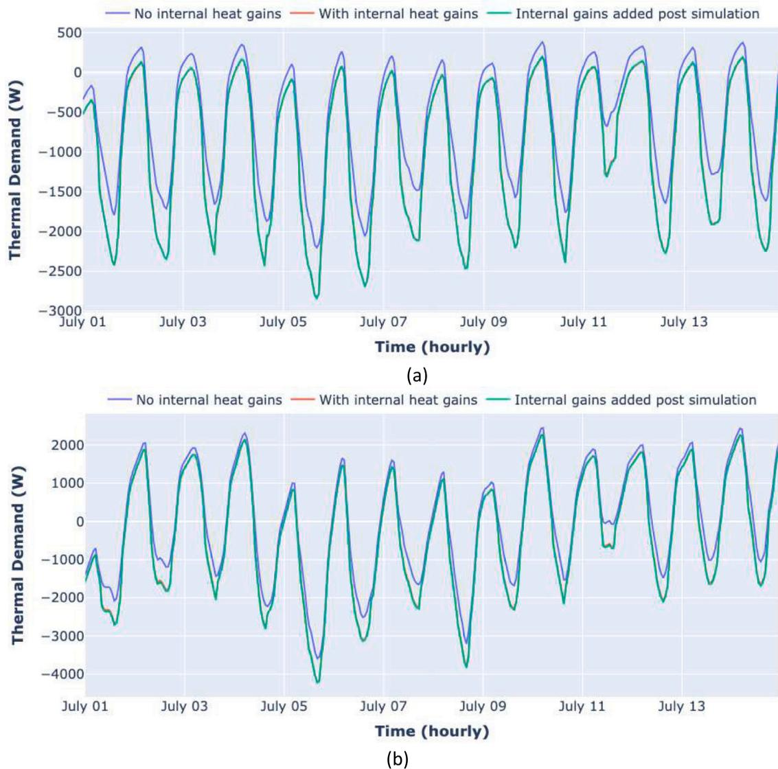
Fig. 23. Effect of internal heat gains in the cooling demand of a detached house in Cardiff oriented at  $0^\circ$  with: (a) the highest thermal efficiency (building code '1111'); (b) the lowest thermal efficiency (building code '7654').
