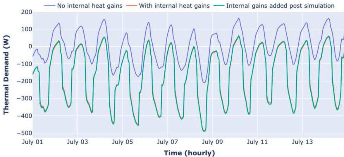
Fig. 21. Effect of internal heat gains in the cooling demand of a ground floor flat in Cardiff with the highest thermal efficiency (building code '1111') and orientation of  $0^\circ$ .
