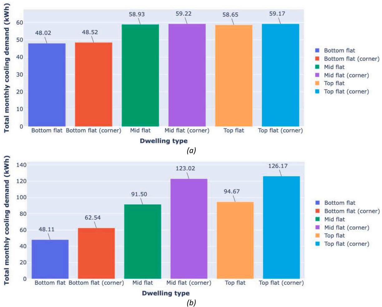
Fig. 13. Total monthly cooling demand in June for all flat types (east-facing external wall, orientation of 90°). Flats with: (a) highest thermal efficiency (building code '1111'), (b) lowest efficiency (building code '7654').
