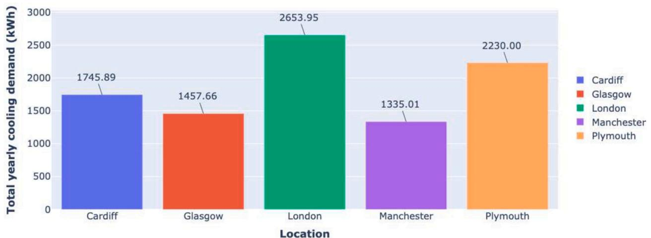
**Fig. 18.** Total yearly cooling demand for a north-facing (orientation of 0°), highly thermally efficient (building code '1111') detached house at different locations in the UK.
