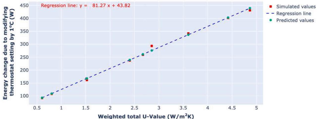
Fig. 6. Variation of hourly thermal demand for a detached house in Cardiff at orientation 0° (i.e. north-facing) for different weighted total U-values.
