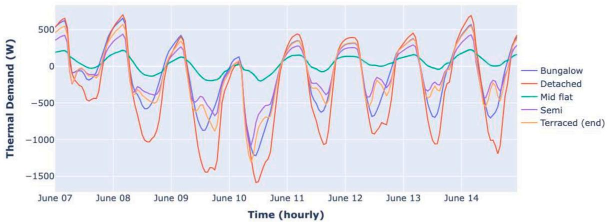
Fig. 11. Hourly cooling demand for each dwelling type in Cardiff with the highest thermal efficiency (building code ‘1111’) and orientation of 0°.
