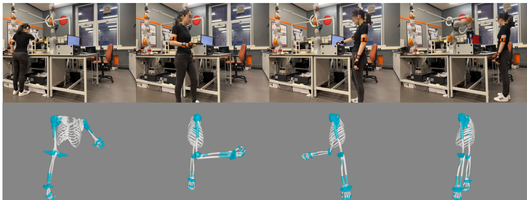
Fig. 8. The process of human-robot collaborative assembly of the desktop PC and its corresponding digital twin human model is depicted from left to right as follows: a human picks up parts in the parts area, transports parts to the assembly area, assembles the parts, and waits for the robot to assemble parts.
