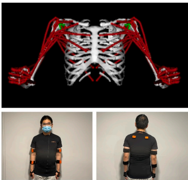
Fig. 3. The upper limb musculoskeletal model and a participant are equipped with Xsens IMU sensors for demonstration.
