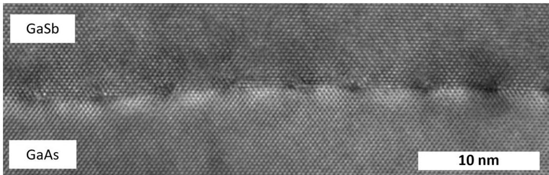
**Fig. 6.22.** High resolution TEM image of the interface between the GaAs and GaSb layers showing the misfit dislocations that form the Interfacial misfit array.
