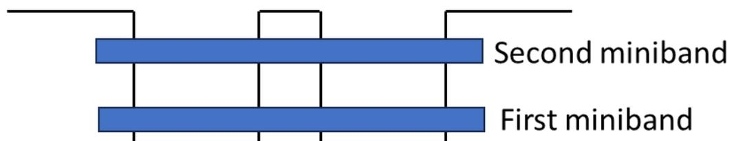
**Fig. 2.10.**  $N$  quantum wells leading to the formation of minibands.
