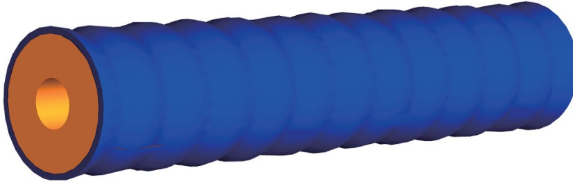
Figure 4. Schematic of the deformed model structure with transverse wrinkles.
