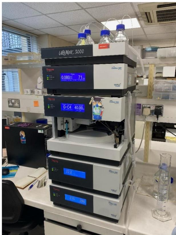
Figure 2-1: Photograph of High-Performance Liquid Chromatography (HPLC) Fractionation Column (Ultimate 3000 nano-LC system) used for the proteomic analyses in this thesis.
