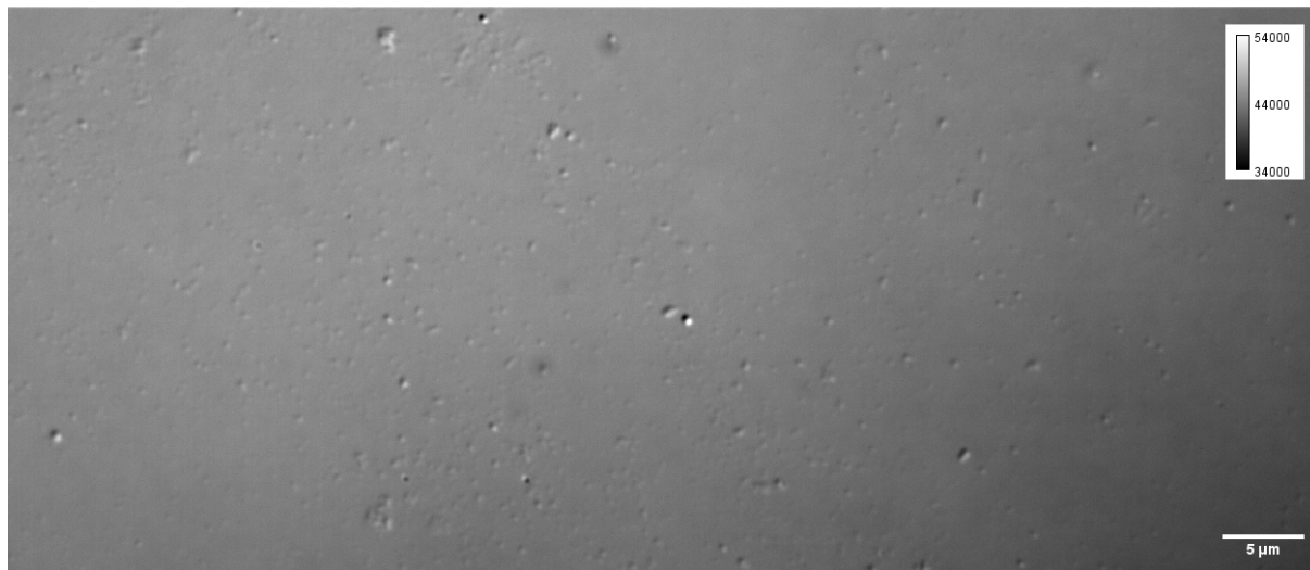
Figure 4.1: Unpurified Honey with Debris and Sugar particles : This transmission DIC image depicts unpurified honey with visible debris and sugar crystals. The sample was prepared by adding 10 \mu L of honey that had not undergone any filtration or refinement processes on a clean coverslip, then covered with a glass slide, highlighting the presence of impurities and unprocessed components within the honey. A 100 \times 1.45 NA oil immersion objective (Nikon MRD01905) and a 1 \times tube lens were used to capture the transmitted light at a polarisation angle \gamma_P = 15^\circ , with 80 ms exposure time, and averaging over 128 frames. A green interference filter (GIF) from Nikon was used to produce light with a peak emission wavelength of 550 nm and blue filter (SchottBG40) was used to cut off infra red wavelength outside the working range of the DIC optical components but detectable on camera. The image size is 1256 \times 541 pixels with a pixel size of 64.1 nm. The image contrast is on a linear grayscale, as indicated.
