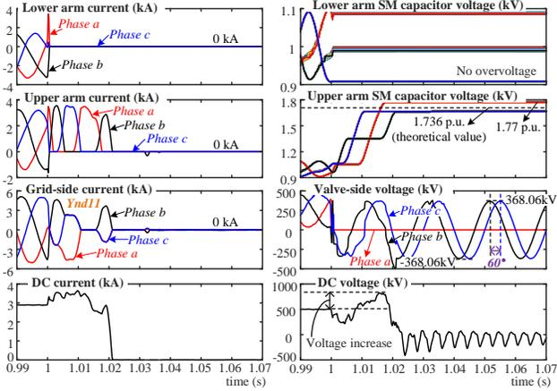
Fig. 11. Simulation results of the MMC with FBSMs.
