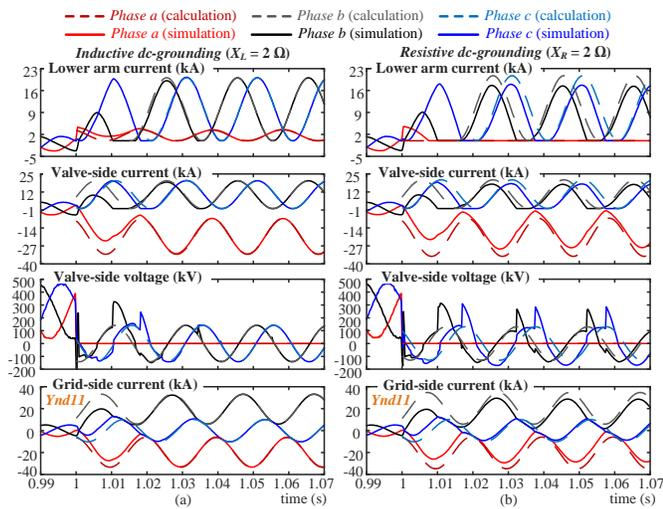
Fig. 14. Comparison between the calculation and simulation results for different dc-grounding methods: (a) inductive dc-grounding, and (b) resistive dc-grounding.
