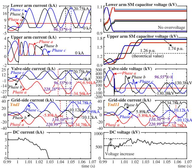
Fig. 10. Simulation results of the MMC with HBSMs under the valve-side SPG fault.
