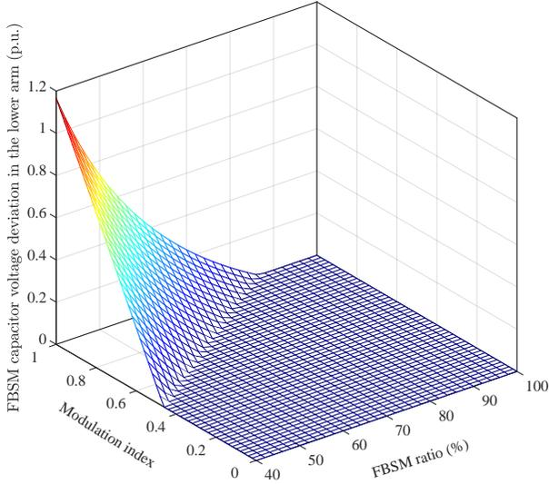
Fig. 7. Overvoltage level in the lower arms of the MMC with hybrid SMs.
