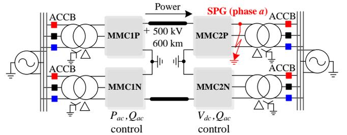
Fig. 9. Bipolar MMC-HVDC test system.
