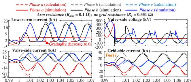
Fig. 15. Comparison between the calculation and simulation results with the inclusion of arm and ac grid resistors.
