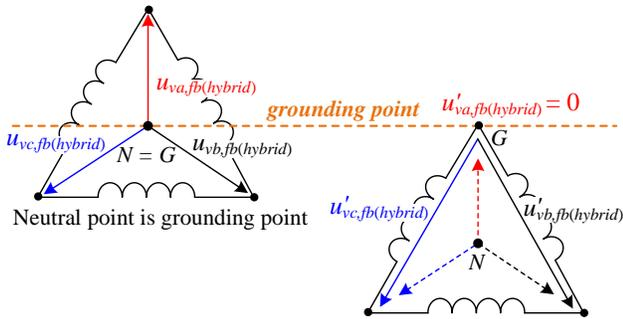
Fig. 6. Valve-side phase voltage under a valve-side SPG fault for the MMC with FBSMs or hybrid SMs.
