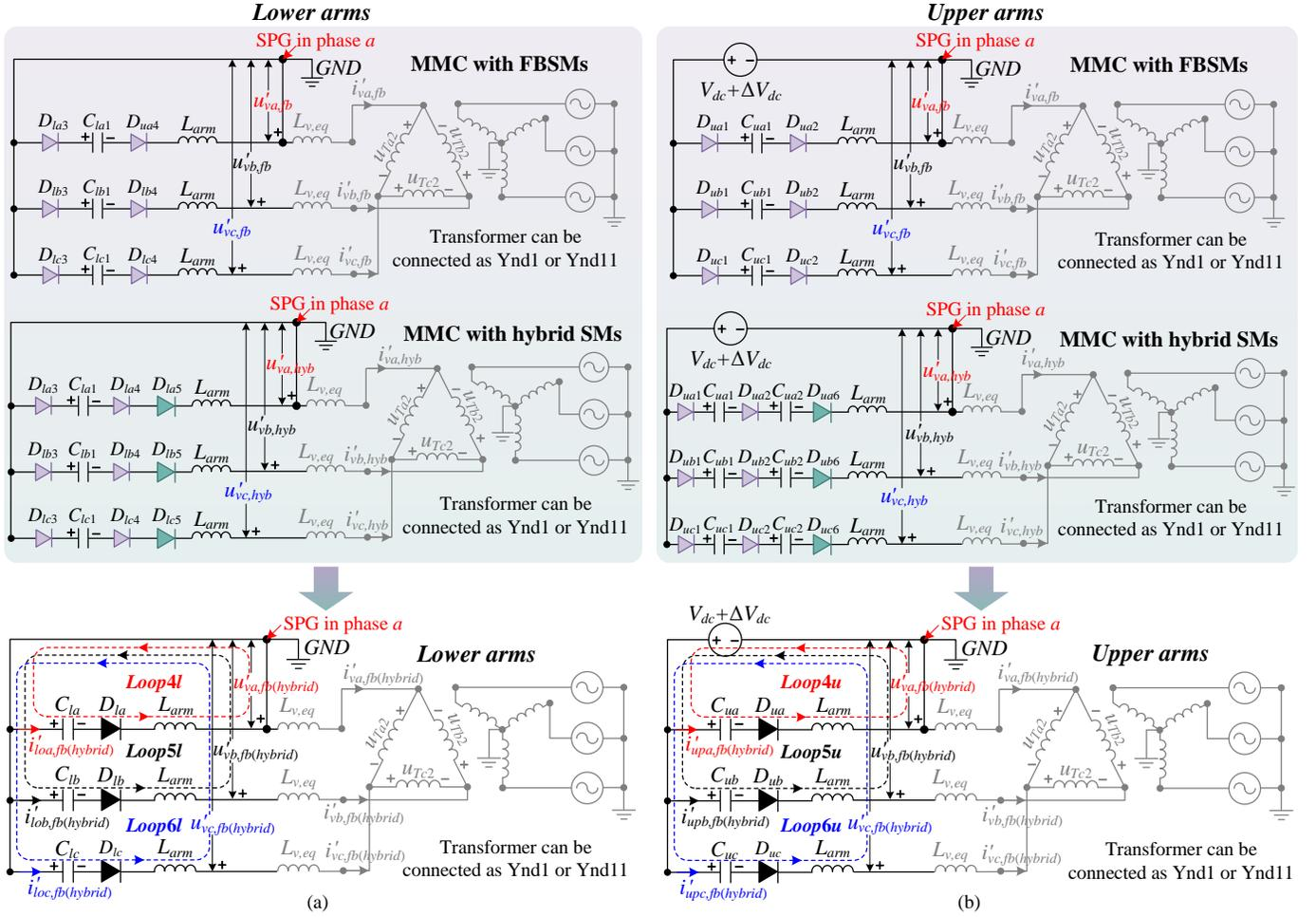
Fig. 5. Equivalent circuits for the MMC with FBSMs or hybrid SMs under a valve-side SPG fault: (a) lower arms, and (b) upper arms.
