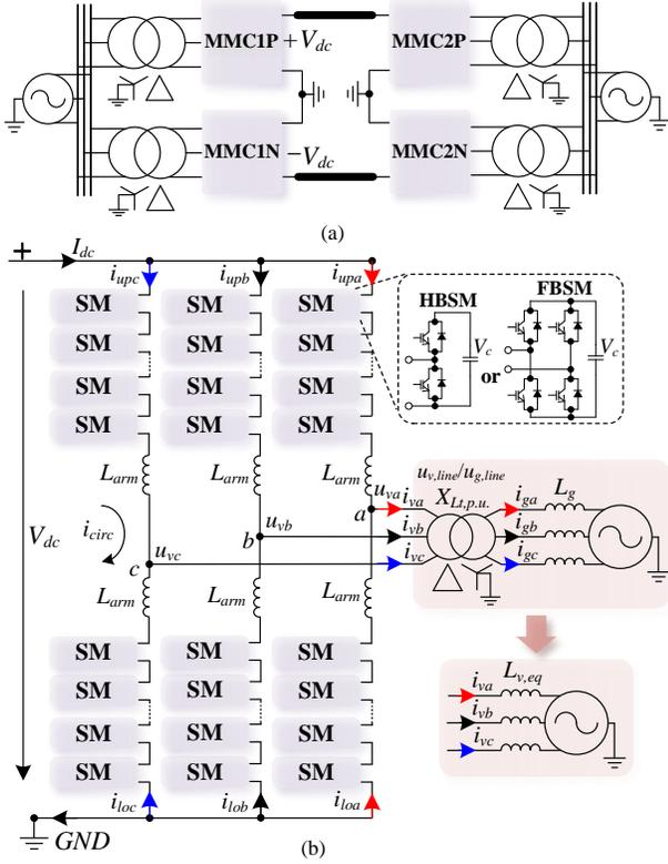
Fig. 1. A bipolar MMC-HVDC link: (a) System diagram, and (b) circuit diagram of the positive pole MMC (MMC1P).
