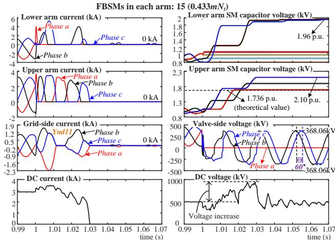
Fig. 12. Simulation results of the MMC with hybrid SMS (15 FBSMs in each arm -  $N_{FB} \approx 0.433mN_t$ ).
