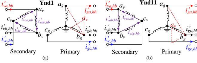
Fig. 4. Transformer wiring configurations: (a) Ynd1, and (b) Ynd11.
