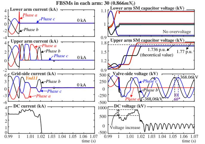
Fig. 13. Simulation results of the MMC with hybrid SMS (30 FBSMs in each arm -  $N_{FB} \approx 0.866mN_t$ ).
