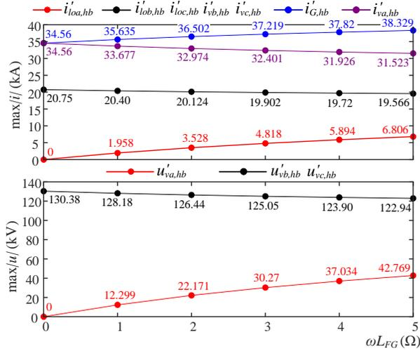
Fig. 8. Post-fault steady-state absolute peak values of lower arm currents, grounding point current, and valve-side currents/voltages with increasing fault-grounding reactance for the HBSM configuration.
