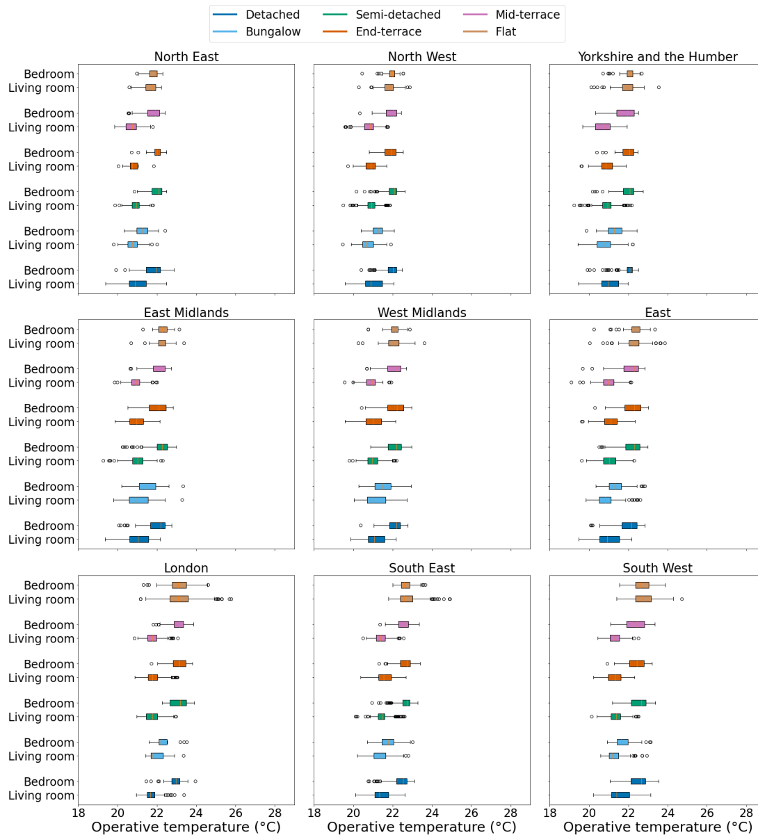
Figure A.9: Daily average mean temperature distribution in living rooms and bedrooms across regions and dwelling types (base climate shutter added).
