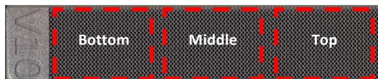
*Figure 5-4. Measurement locations of strut analysis*
