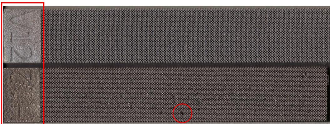
Figure 5-2. Example of dislocated struts on sample H12 (bottom) compared to V12 (top), where the large dislocation (circle) is shown and the differing colours highlighted on the labels (square).
