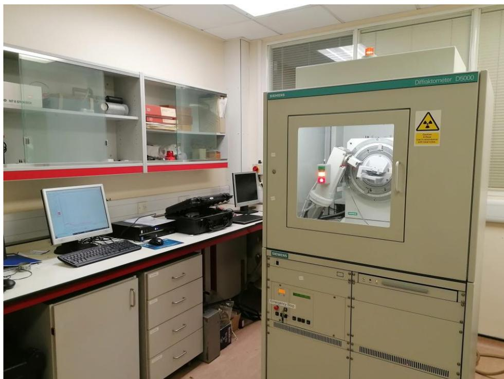
Figure 3-11 Siemens D5000 X-ray diffractometer system.
