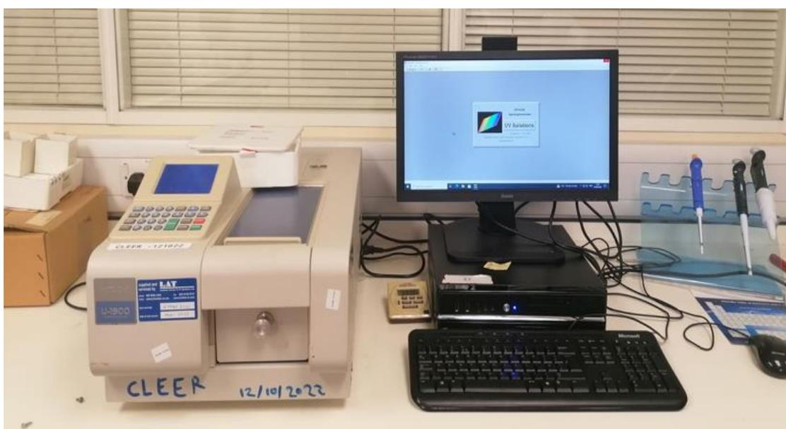
Figure 3-8 Hitachi U-1900 Spectrophotometer
