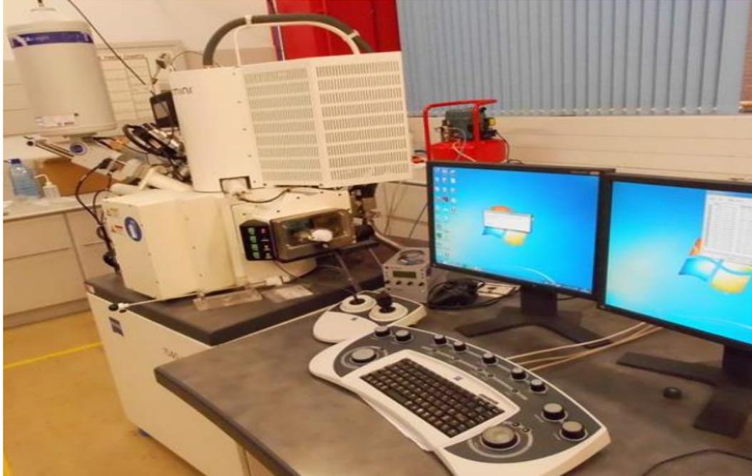
Figure 3-14 Zeiss 1540 XB Crossbeam Field emission scanning electron microscope (FE-SEM)
