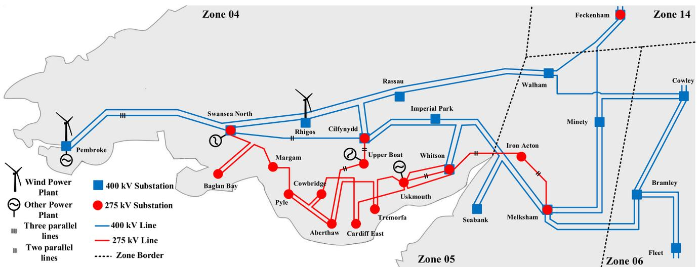
Fig. 5. Configuration of the south Wales and west England transmission network in 2030. This figure was produced using data from [46–48].
