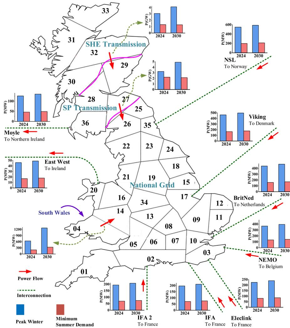
Fig. 4. Power flow dynamics across GB and interconnections under peak winter and minimum summer demand conditions for 2024 and 2030
