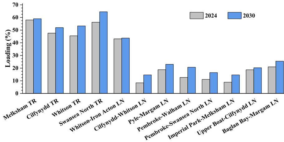
Fig. 6. Loading characteristics of selected lines and transformers in south Wales during peak hour.
