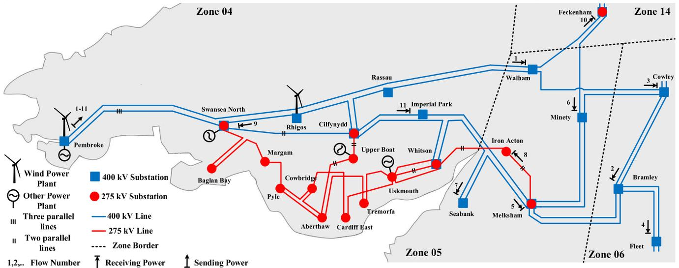
Fig. 12. Power exchange results for Pembroke-Walham line based on FDT during peak hour in South Wales, and west of England.
