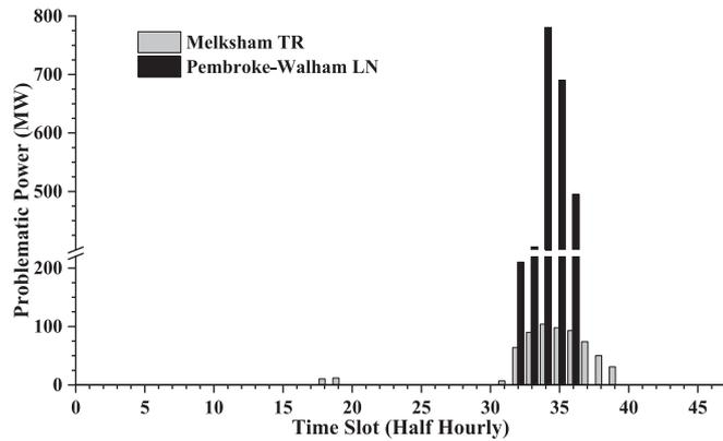
Fig. 14. Problematic power for Pembroke-Walham line and Melksham transformer.
