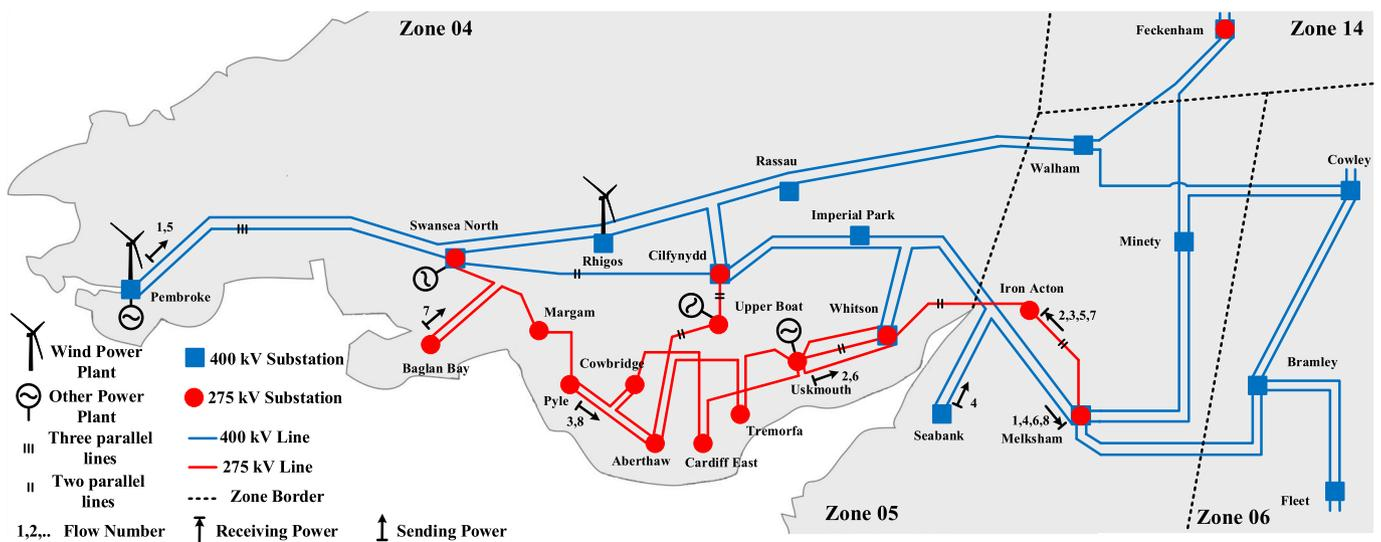
Fig. 13. Power exchange results for Melksham transformer based on FDT during peak hour in South Wales, and west of England.
