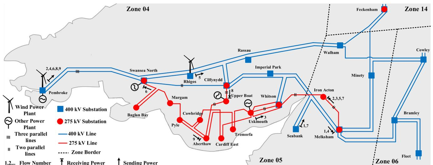
Fig. 8. Power exchange results for Melksham transformer based on FDT during peak hour in south Wales, and west of England.
