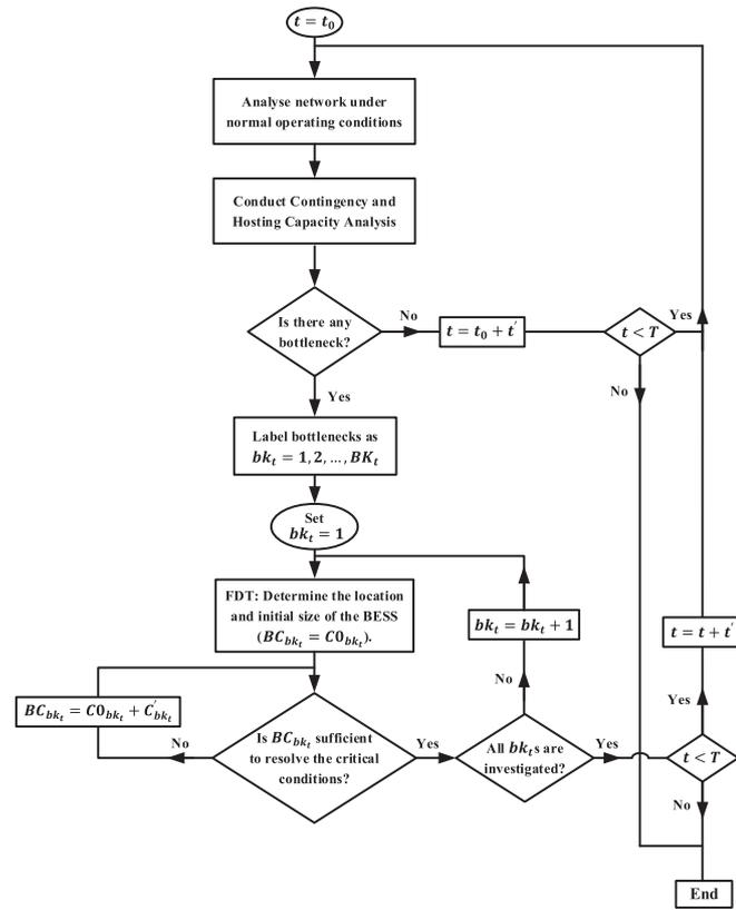
**Fig. 9.** Flowchart for determining size and location of BESSs to address the network bottlenecks.
