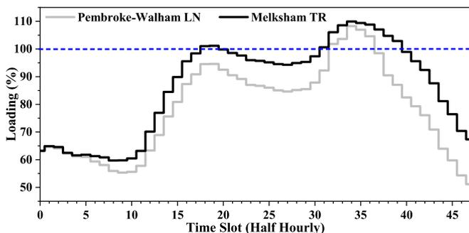
Fig. 11. Loading of the Pembroke-Walham line and Melksham transformer under N-1 contingency on peak winter 2030.
