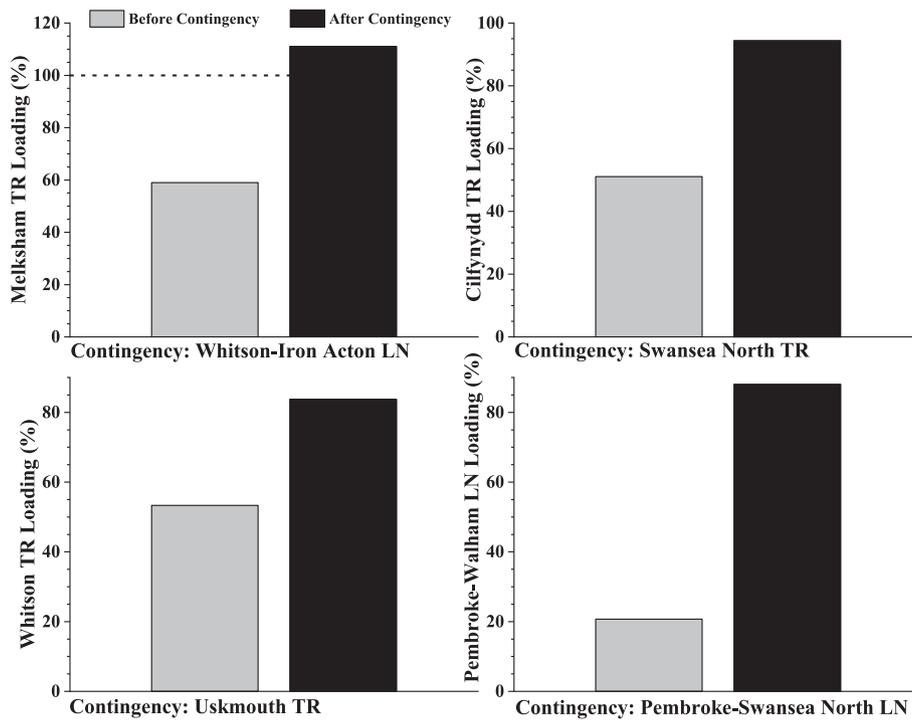
Fig. 7. Results of N-1 contingency analysis in south Wales during peak hour.
