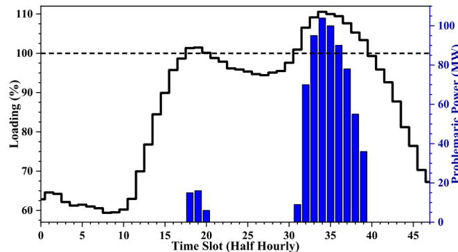
**Fig. 10.** Loading and problematic power of the Melksham transformer under N-1 contingency on peak winter 2030.
