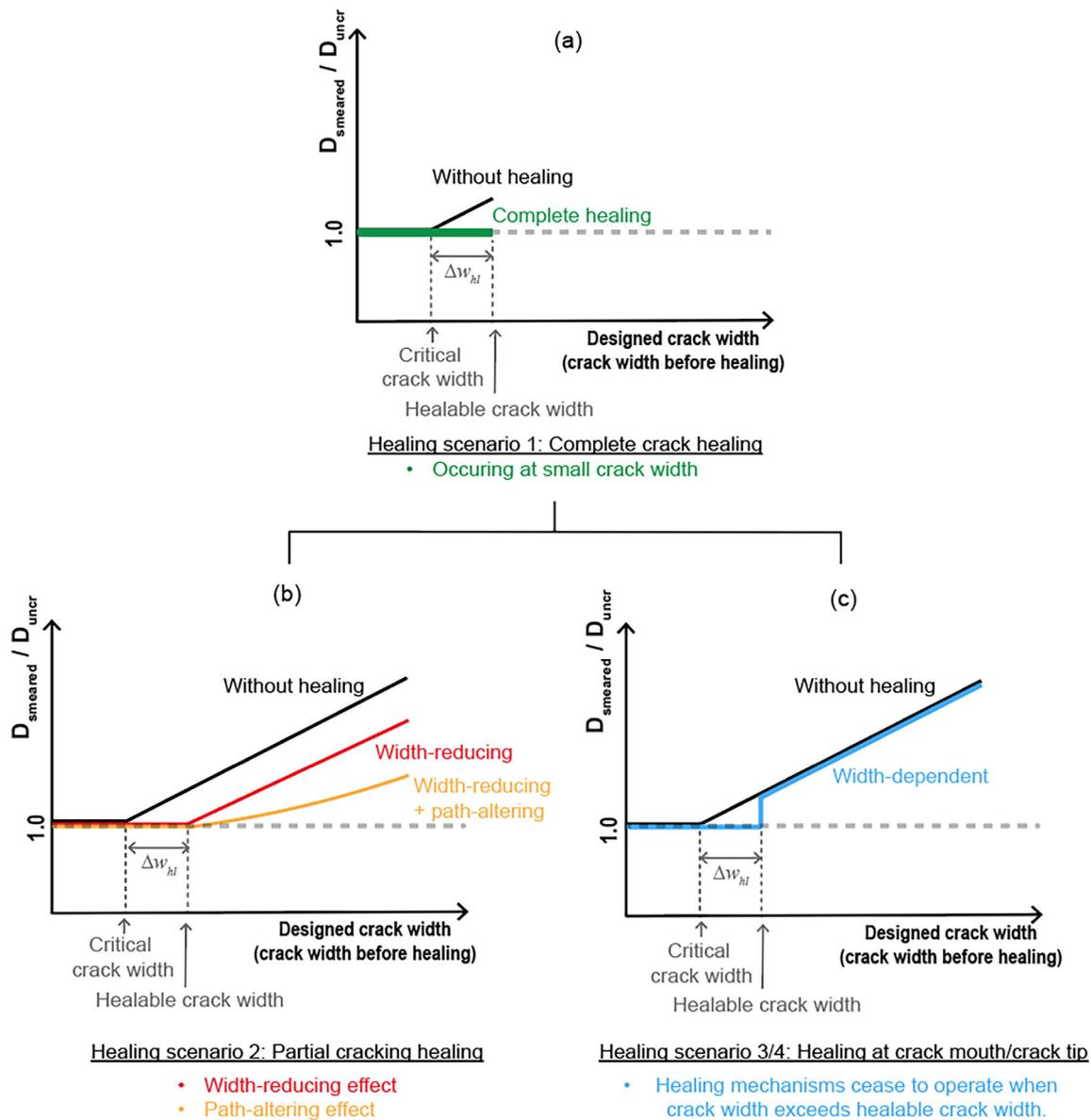
**FIGURE 3** Schematic illustration of the relationship between diffusion coefficient and crack width for (a) complete healing, (b) partial healing, and (c) healing methods functioning only at small crack widths for rapid healing.
