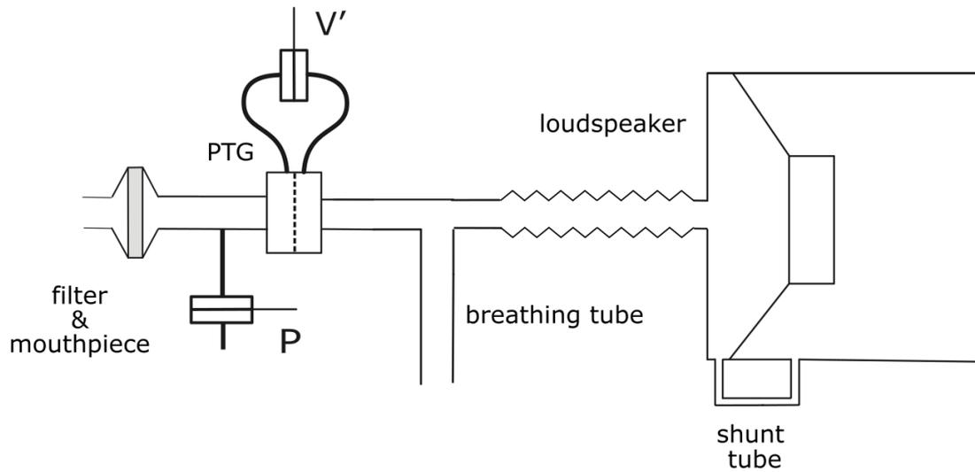
**Figure E1.** Schematic arrangement of the oscillometry device. PTG: pneumotachograph; pressure (P) and flow (V') sensors: Honeywell model 26PCAFA6D (Golden Valley, MN, USA). Antibacterial filter with mouthpiece (Microgard-II microbial filter, Vyair, Germany).
