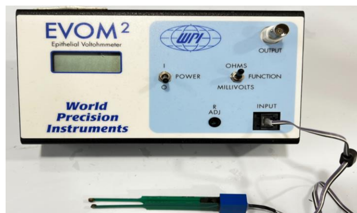
Figure 2.14 EVOM 2 Epithelial Volt/Ohm Meter with chopstick electrode for measuring the resistance between the two electrodes (World Precision Instruments, Hitchin, Hertfordshire, UK).
