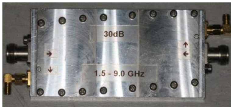
Figure 3.11 Microwave directional coupler used in this research (Ehtaiba 2017)
