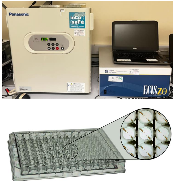
Figure 2.12 The ECIS instrument and ECIS microarray used in the present.
