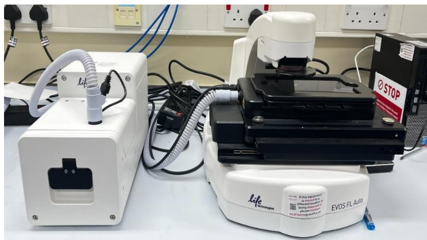
Figure 2.8 EVOS® FL2 Auto Imaging System with EVOS® Onstage Incubator, which provide the environment condition at 37°C, 5% CO 2 for cells, and capture the cells via the various zoom of microscope.
