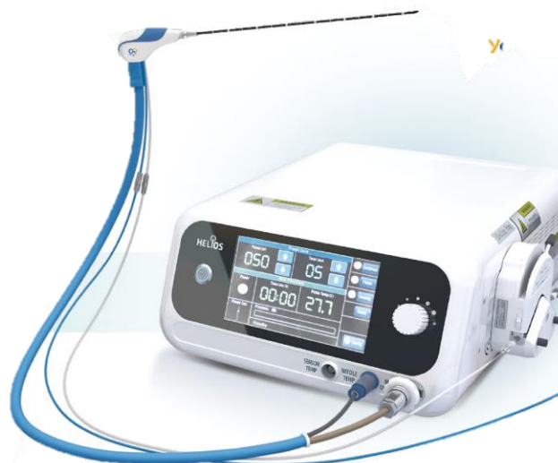
Figure 1.7 Percutaneous microwave ablation. (A) The schematic diagram of PMA. The applicator is places percutaneously into the tumour mass before microwave energy is applied to heat the tumour (Brace 2010). (B) Current clinical PMA device. Available: https://www.keymax.com.hk/products/helios-microwave-ablation-system-h-1
