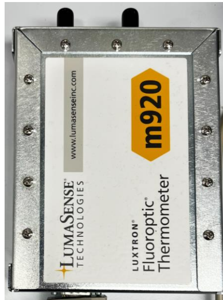
Figure 3.16 Luxtron M922 Fiber Optic Temperature Sensor.
