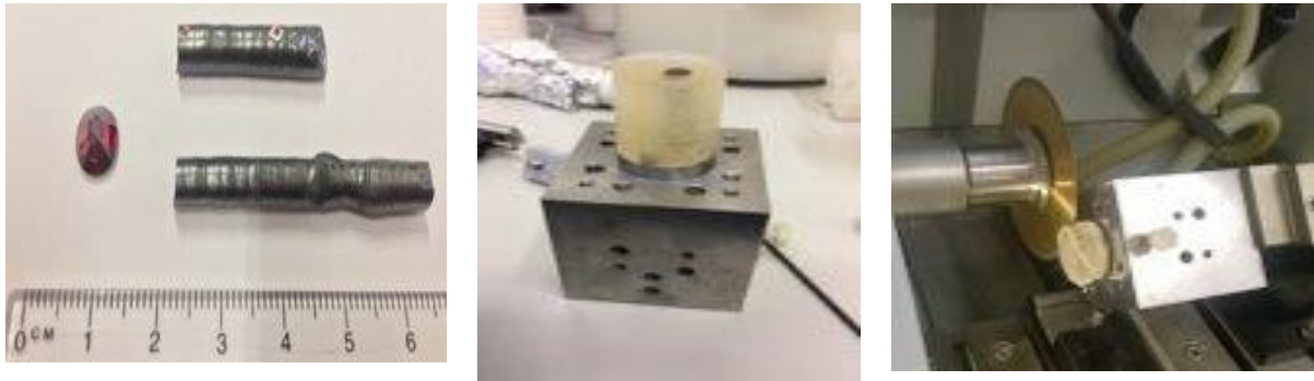
Figure 3.1: (a) Cu 2 O material initially in bar form. (b) The sample securely embedded in resin for processing. (c) Abrasive wet cutting process using a precision diamond saw to achieve smooth, undistorted surfaces essential for further preparation.
