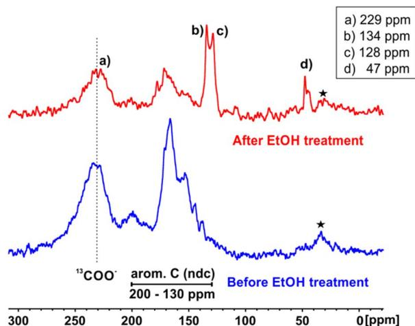
Fig. 8 Solid-state NMR spectra of pristine  $^{13}\text{C}$ -DUT-8(Ni) sample (blue) and sample treated with  $^{13}\text{C}$ -labelled ethanol (red). The signals marked with an asterisk are rotational sidebands of the signal at 240 ppm.
