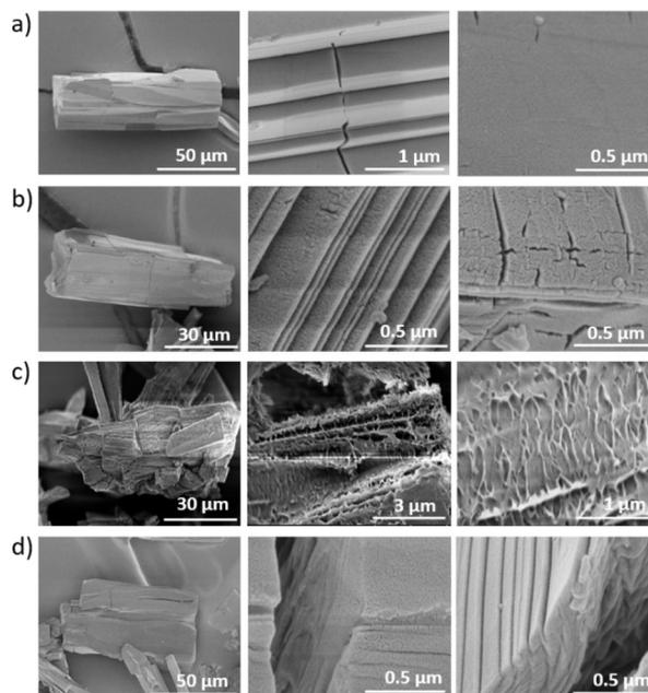
Fig. 3 SEM images of (a) pristine DUT-8(Ni) sample and treated samples (b) 2\_EtOH-6, (c) 3\_EtOH/H<sub>2</sub>O, (d) 4\_PDMS.
