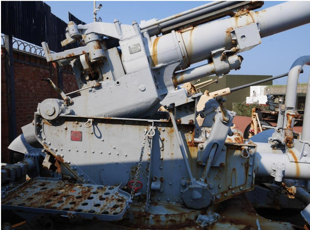
*Figure 2.5: One of English Heritages' 3.7-inch AA gun, on loan at Heugh Battery, Hartlepool, an exposed coastal location showing, signs of corrosion around panel joints*
