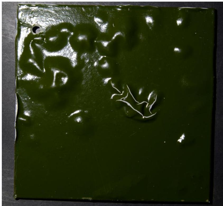
*Figure 7.4: Examples of surface blistering across a Hempel sample after 9 months of ageing*
