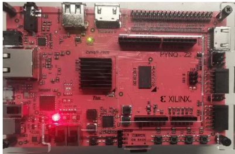
**Figure 6.8 Xilinx PYNQ-Z2 platform for data processing in the experiment.**
