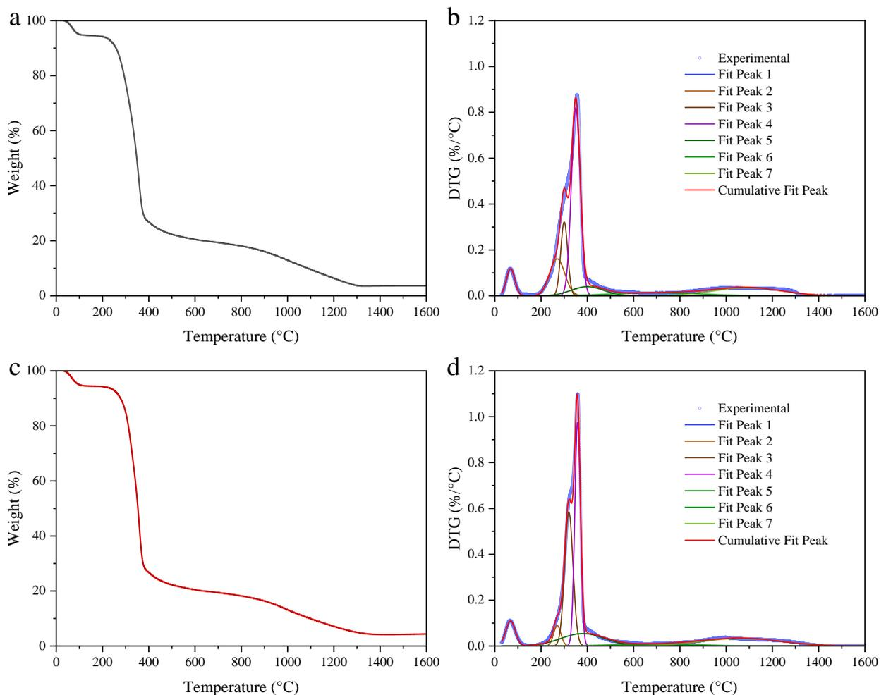
Figure 5-7. TGA curves and the gauss peak fitted experimental DTG curves of (a and b) Ash and (c and d) Larch samples.
