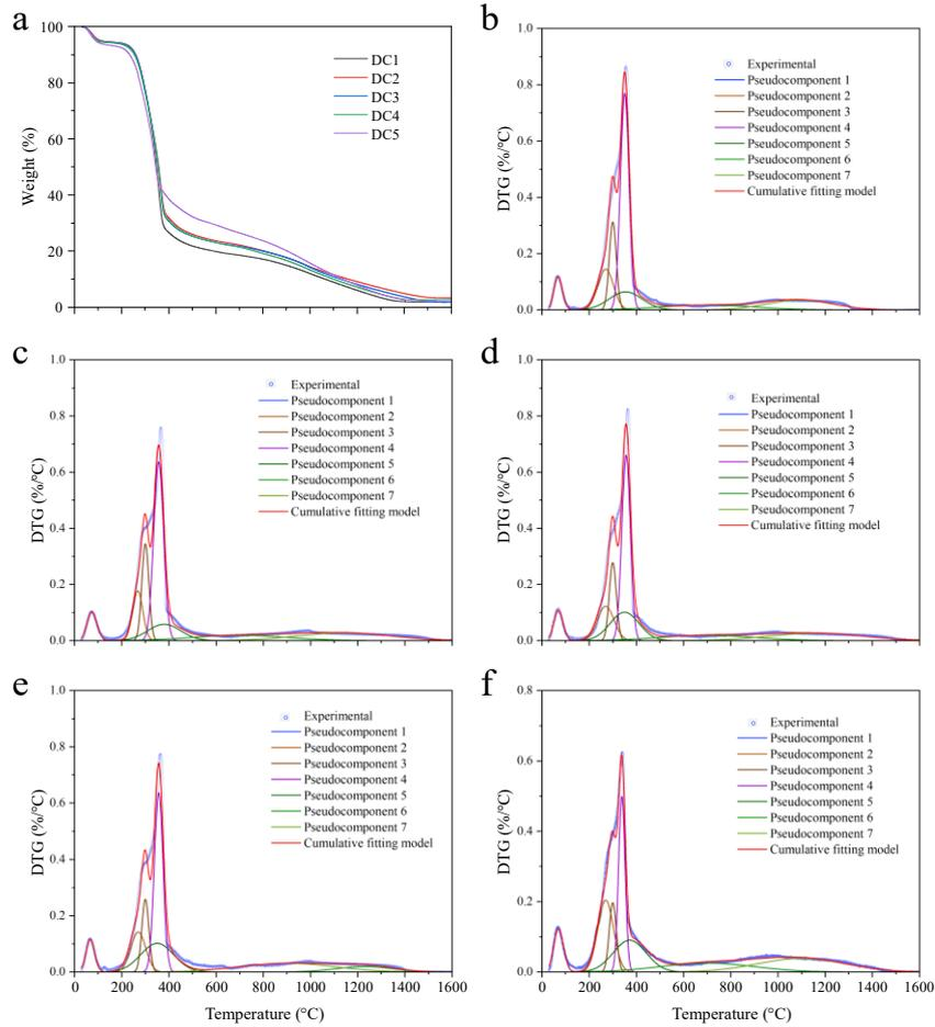
Figure 4-4. (a) TGA curves comparison of Ash wood samples from five decay classes. The gauss peak fitted experimental DTG curves, (b) DC1; (c) DC2; (d) DC3; (e) DC4; (f) DC5.
