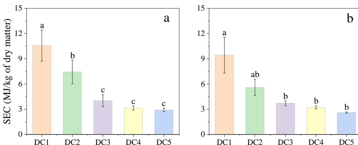
Figure 4-1. Specific energy consumption (SEC) for grinding wood samples from five decay classes, (a) Birch; (b) Ash. Different lowercase letters above each column indicate significant differences (columns with different letters are statistically significantly different from one another).
