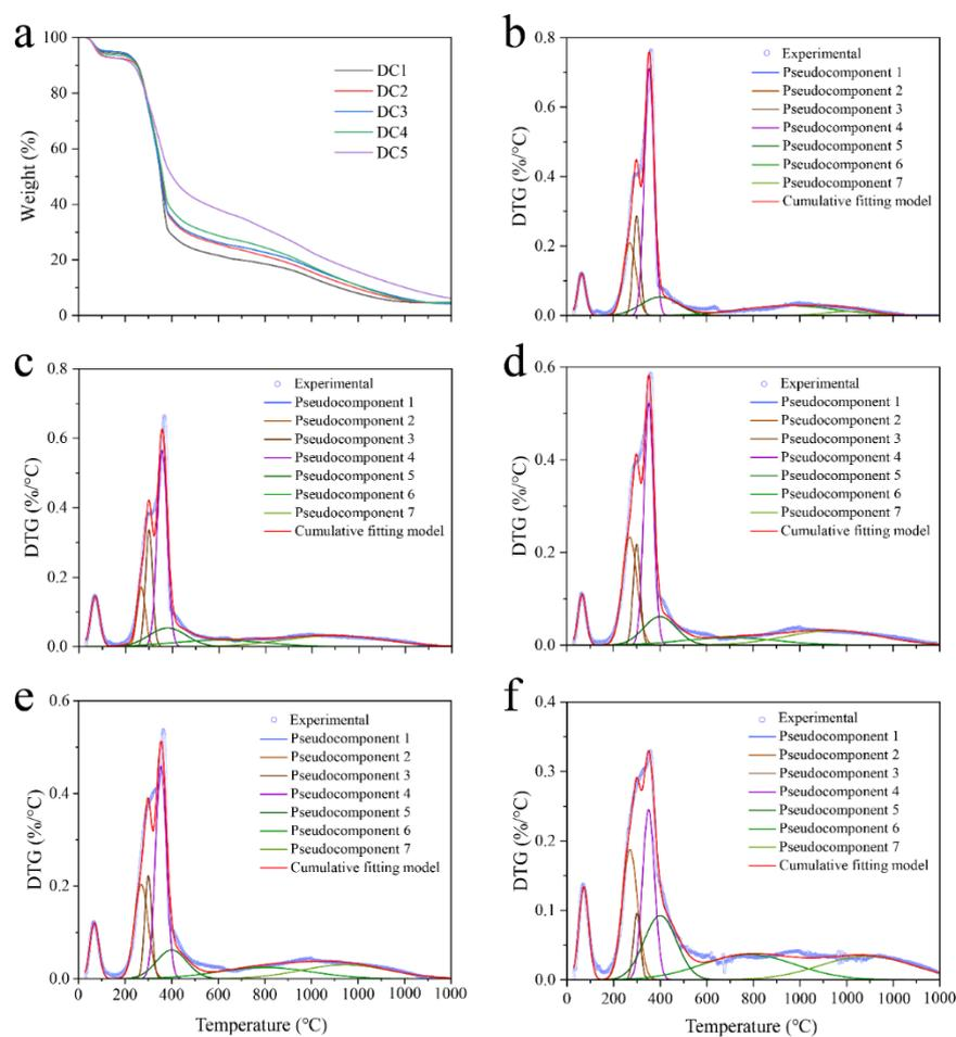
Figure 4-3. (a) TGA curves comparison of Birch samples from five decay classes. The gauss peak fitted experimental DTG curves, (b) DC1; (c) DC2; (d) DC3; (e) DC4; (f) DC5.
