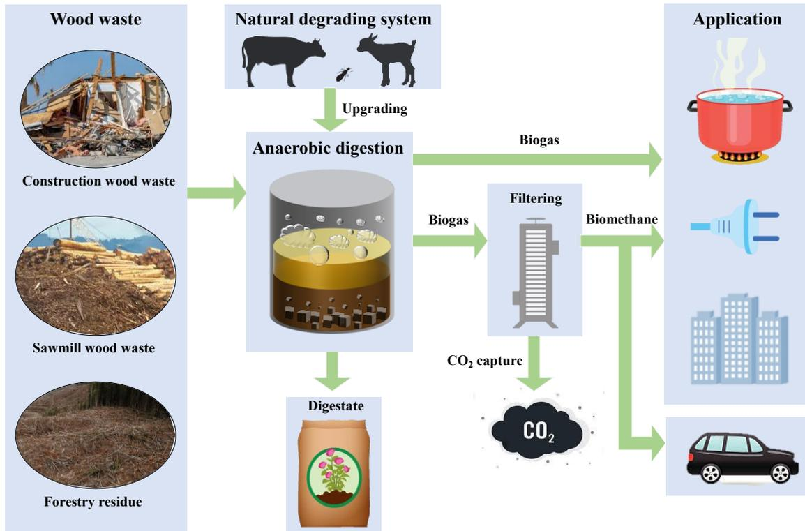
Figure 2-8. Schematic diagram of biogas production pathways from different kinds of wood wastes.
