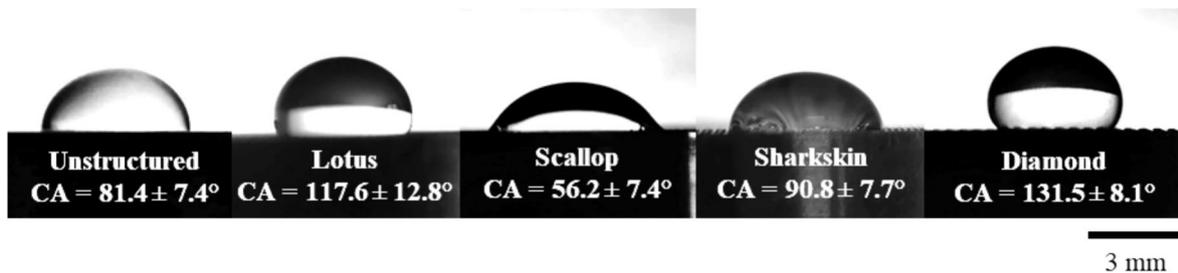
**Fig. 10** Contact angles between water droplets and the textured and untextured surfaces
