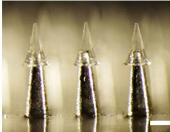
Figure 2-3 - Biodegradable MN design with an arrowhead design are shown. The arrowhead breaks off into the skin where the polymer and encapsulated drug dissolves into the blood stream over a set period of time [41]
