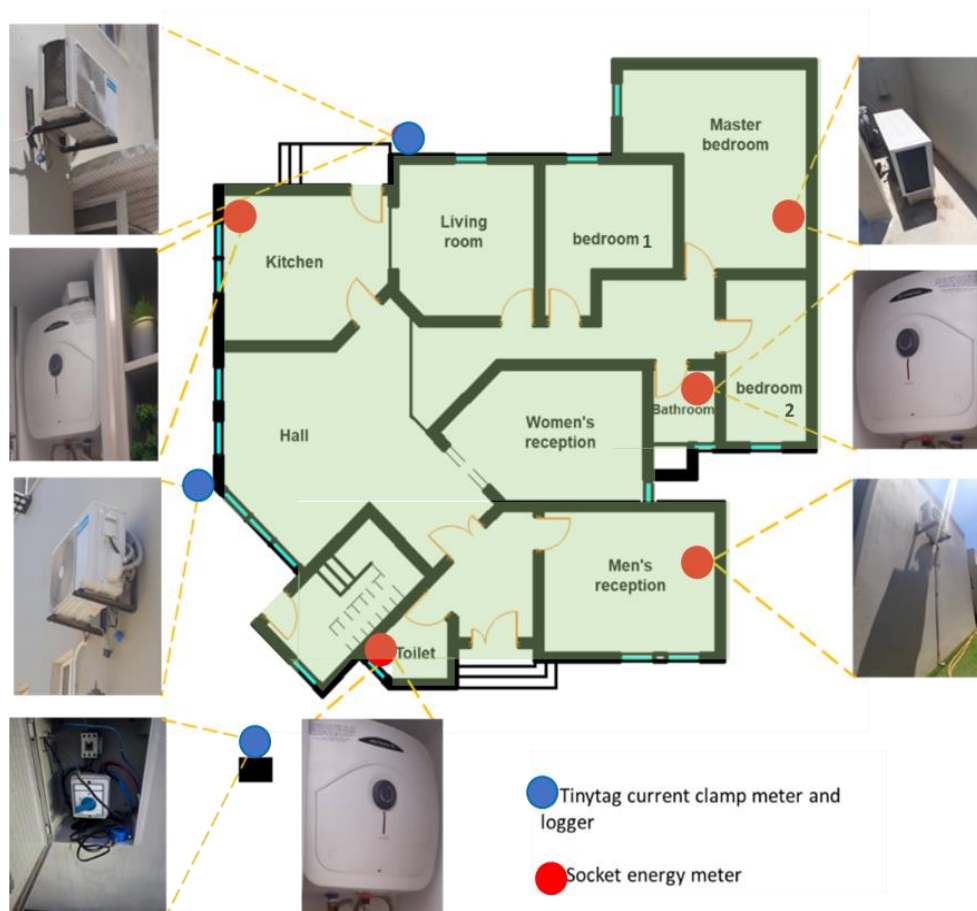
Figure 4. 19 Energy meter locations and installation for Case Study 2
