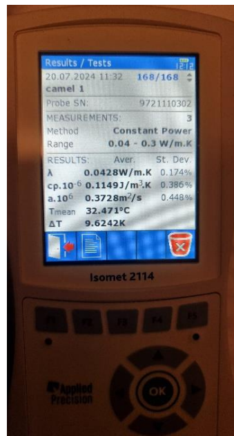
Figure 4. 25 The thermal conductivity of camel hair, measured by ISOMET 2114
