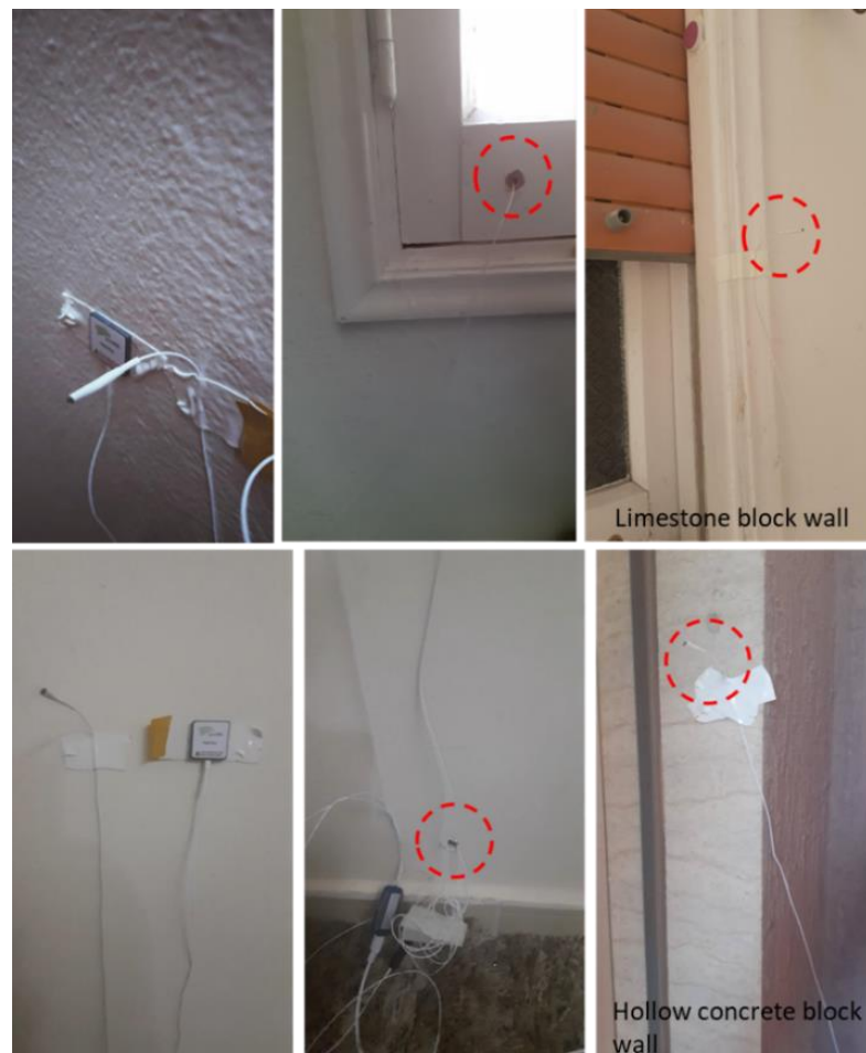
Figure 4. 16 Heat flux sensor installation on both the limestone block wall and hollow concrete block wall
