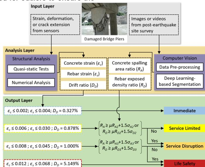
Figure 1: Hybrid Structural-Vision Damage Evaluation Framework.
