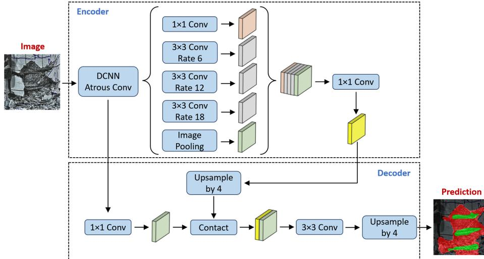
Figure 3: The structure of Deeplabv3+.
