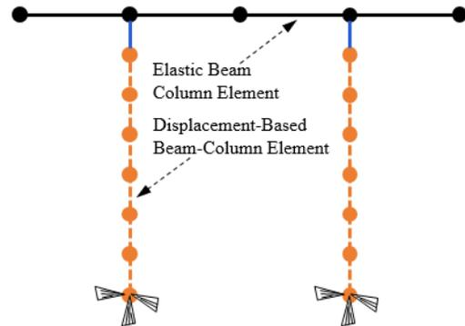
Figure 2: RC Double-column pier modelling information.
