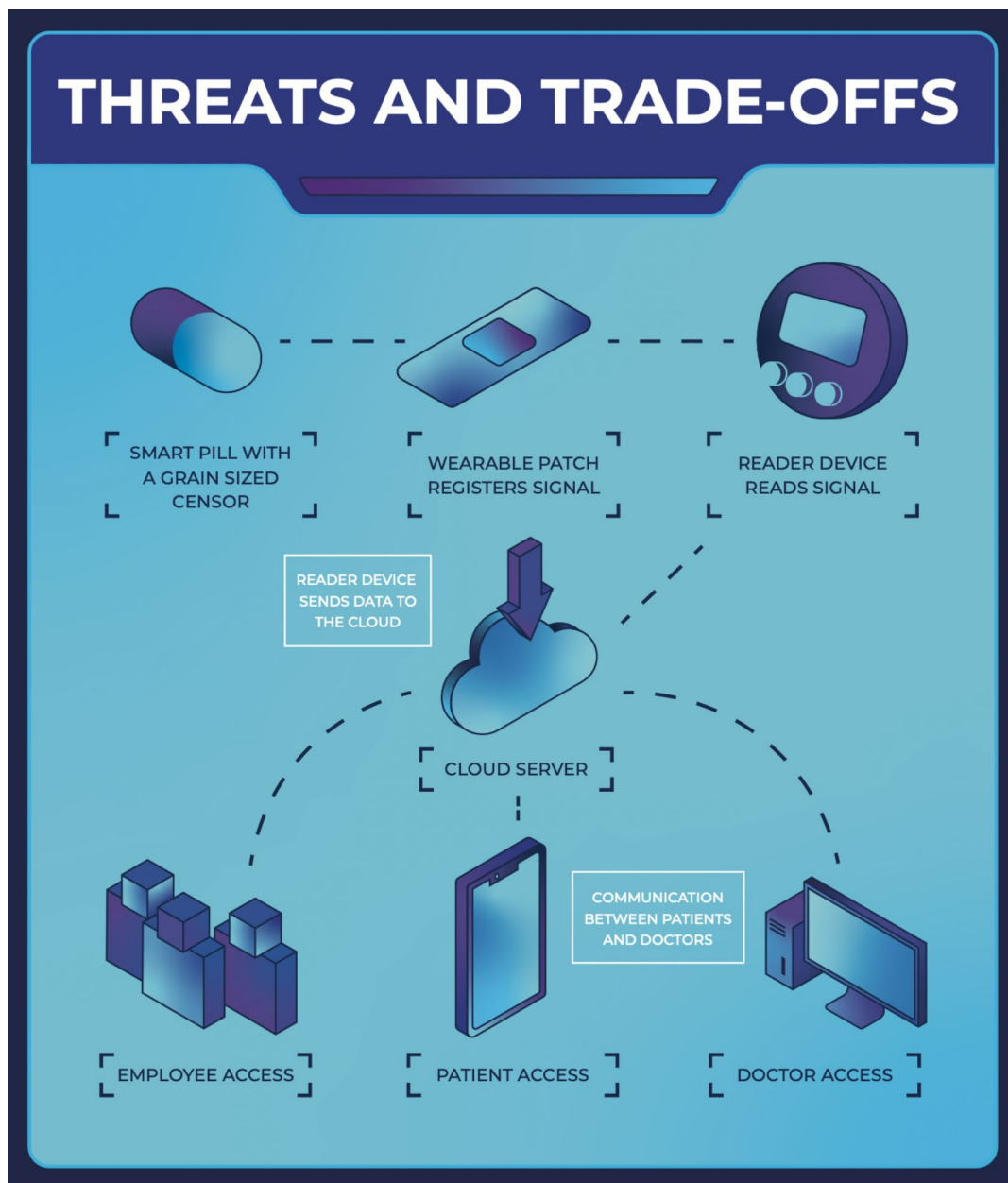
Fig. 1 The premise of the game: the dataflow diagram of a connected digital healthcare system
