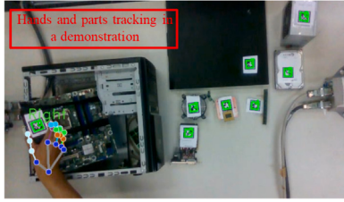
Fig. 6. The top-down view illustrates the demonstration of the desktop assembly process by a human operator. A visual method is used for tracking both the hands and the parts. Action and state recognition are performed using the method in You et al. (2022).
