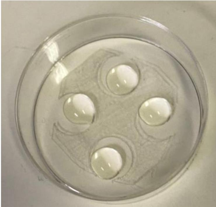
**Figure 2.10: Open samples for protein insertion** An image to show the set up of the open samples with droplets applied ready for imaging in a plastic dish with a 35 mm diameter
