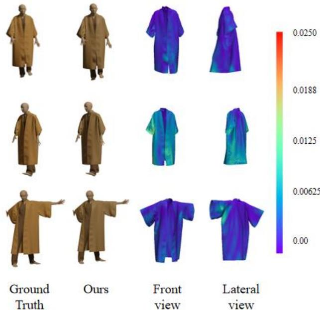
**FIGURE 3** Examples of our MGN for garment deformation in different pose. The first column is the ground truth generated by physics-based simulation. The second column is the results obtained by MGN. Our method can produce natural and realistic clothing dynamics. The third column and the fourth column represent the vertex deviations from the front view and the side view, respectively. Colder colors indicate smaller errors.
