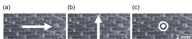
Fig. 12. The three sample orientations relative to the microwave E -field in the TM_{010} cavity, showing the main orientation of the SiC fibre tows that run the full length of the CMC samples. All measurements of environmental damage are in (b), the perpendicular sample orientation, with a 5.1 mm cavity gap to allow the sample to be inserted and removed easily.
