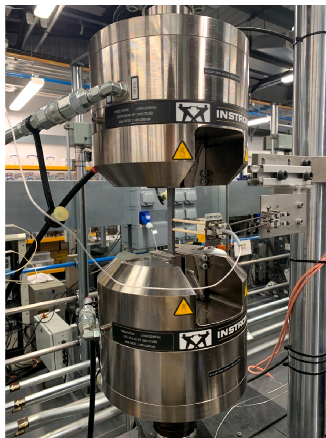
Fig. 11. Tensile test setup using 12.5 mm gauge extensometer.
