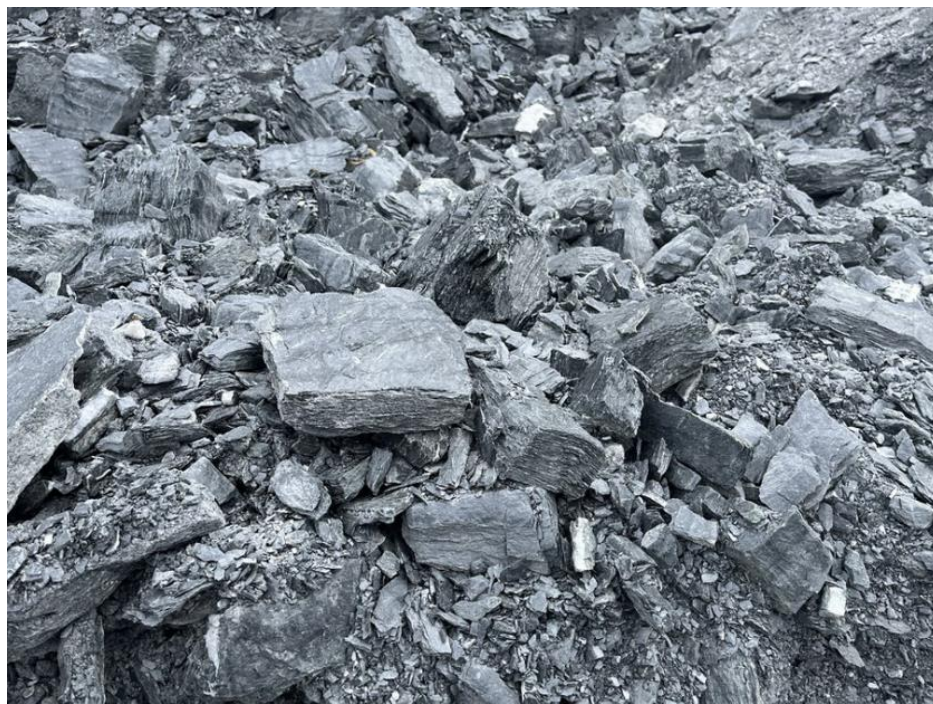
Fig. 1. Weathered phyllite filler studied.
