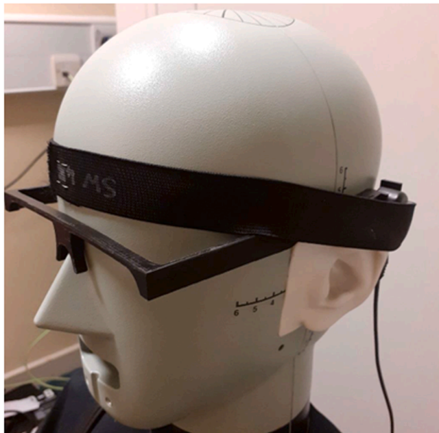
Fig. 2. Transducer mounting for the unimpaired participants, featuring 3D-printed spectacle frames that hold the bone vibrator against the temporal bone and an elastic strap to maintain pressure.
