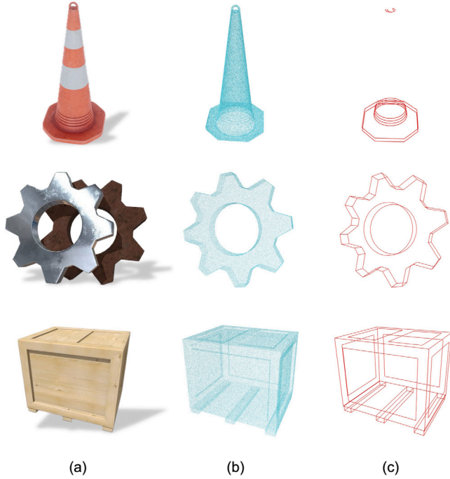
Fig. 20. Feature extraction results from uniform real-world scanned point clouds. (a) Real-world objects; (b) scanned point clouds; (c) extracted feature lines.
