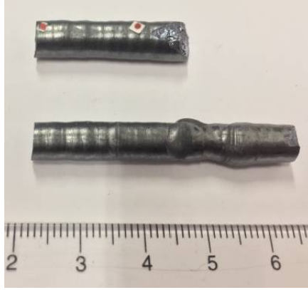
Figure 3.1: Rods of \text{Cu}_2\text{O} grown using the optical floating-zone method. Thin discs were cut from the rods to prepare the samples that were used.
