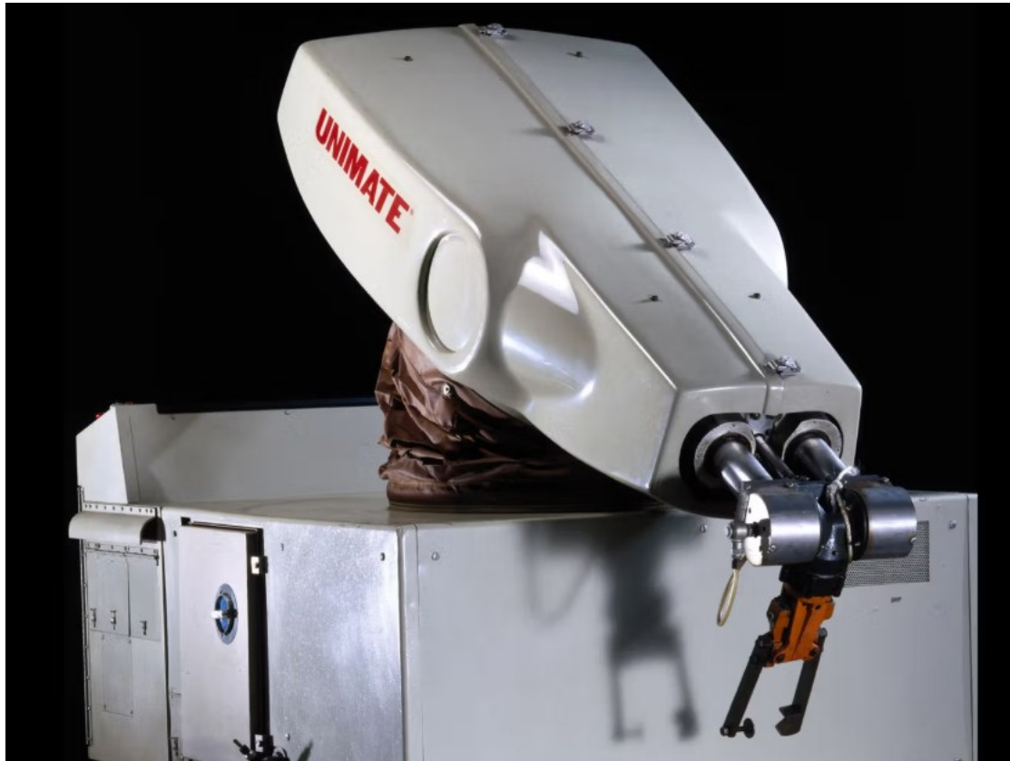
Figure 2.3 Unimate robot. Source: (IEEE, 1961).
