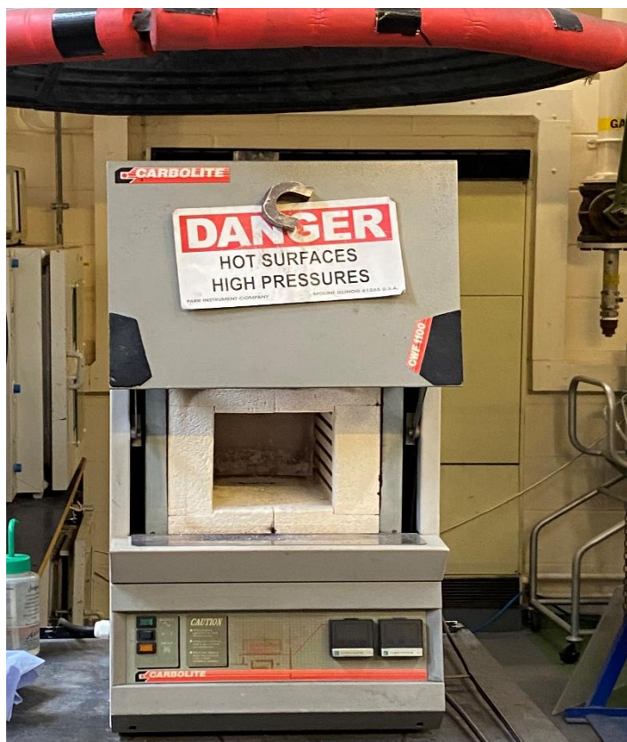
Figure 3.9: Muffle furnace, Carbolite furnace used for volatile matters and ash content measurement.
