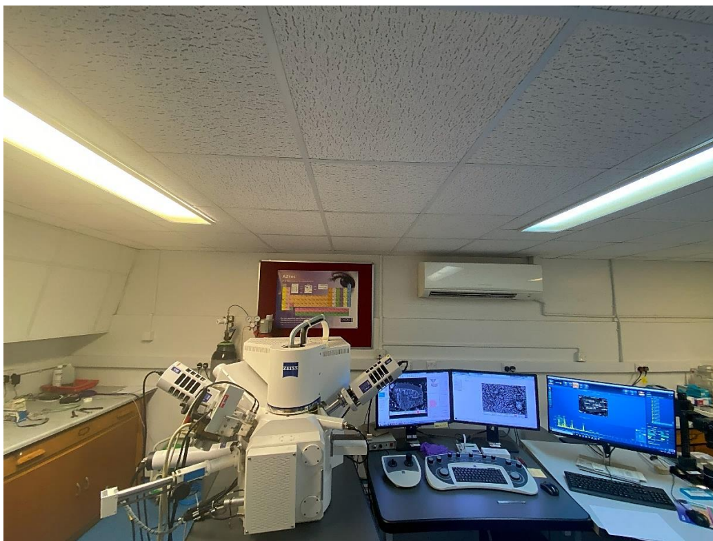
Figure 3.24: Zeiss SIGMA HD VP Field Emission Scanning Electron Microscopy system used for SEM-EDS analysis.
