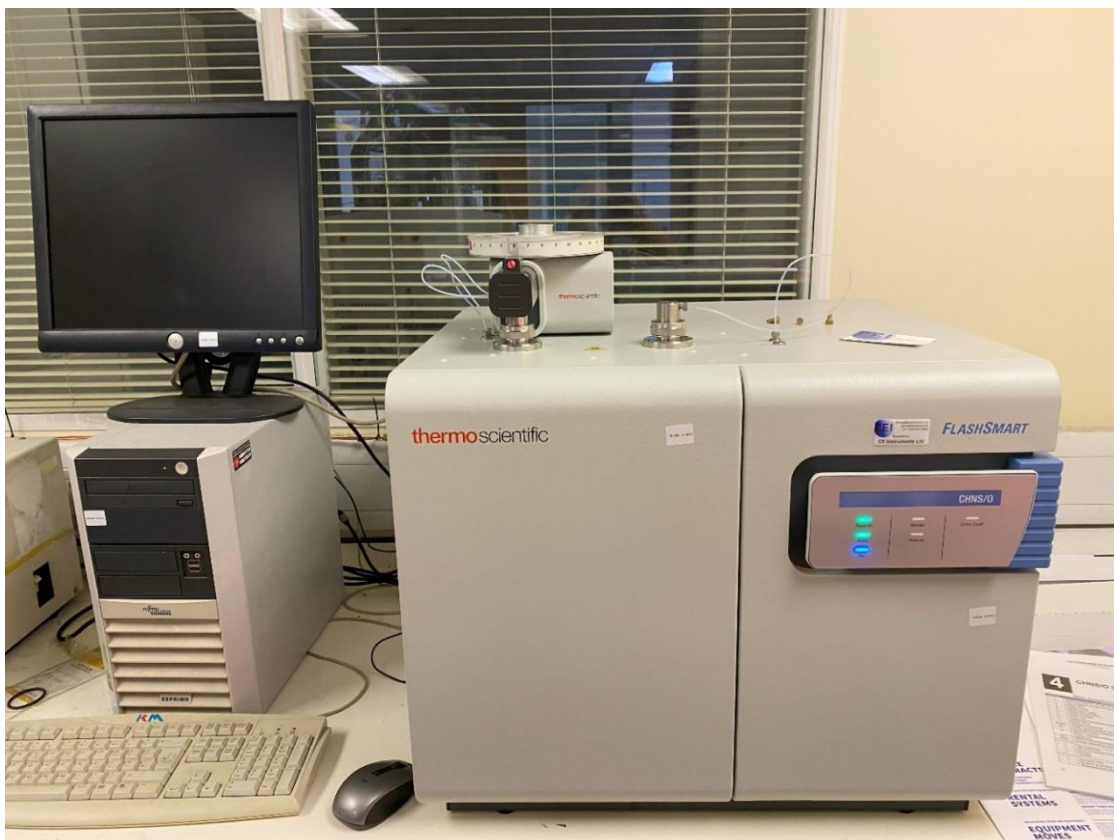
Figure 3.10: Thermoscientific FlashSmart Organic elemental analyser (OEA), CHNS/O for Ultimate analysis.
