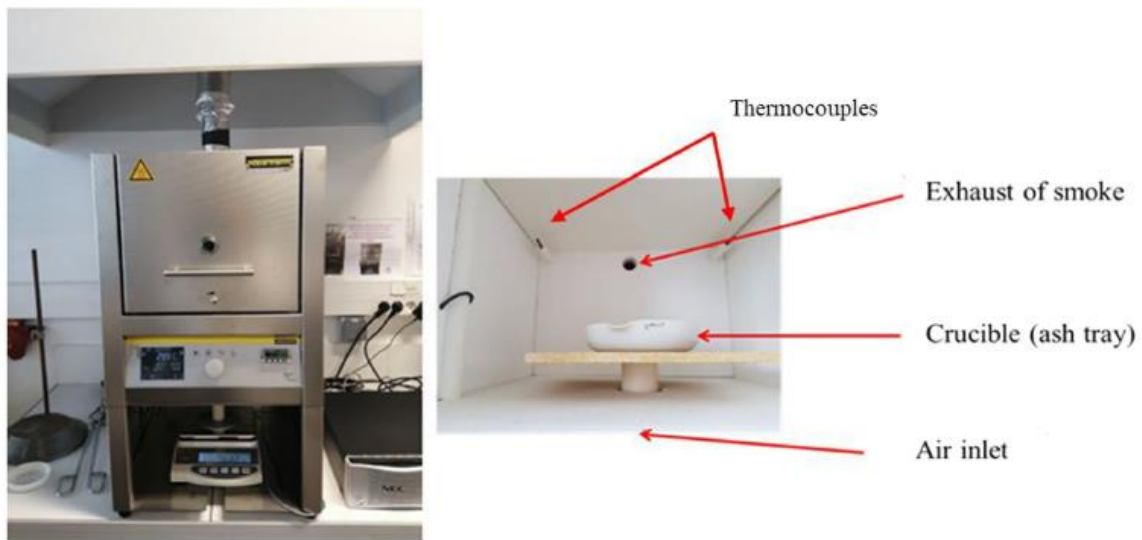
Figure 2.10: Macro-TGA system with high temperature furnace developed by Nabertherm [79].
