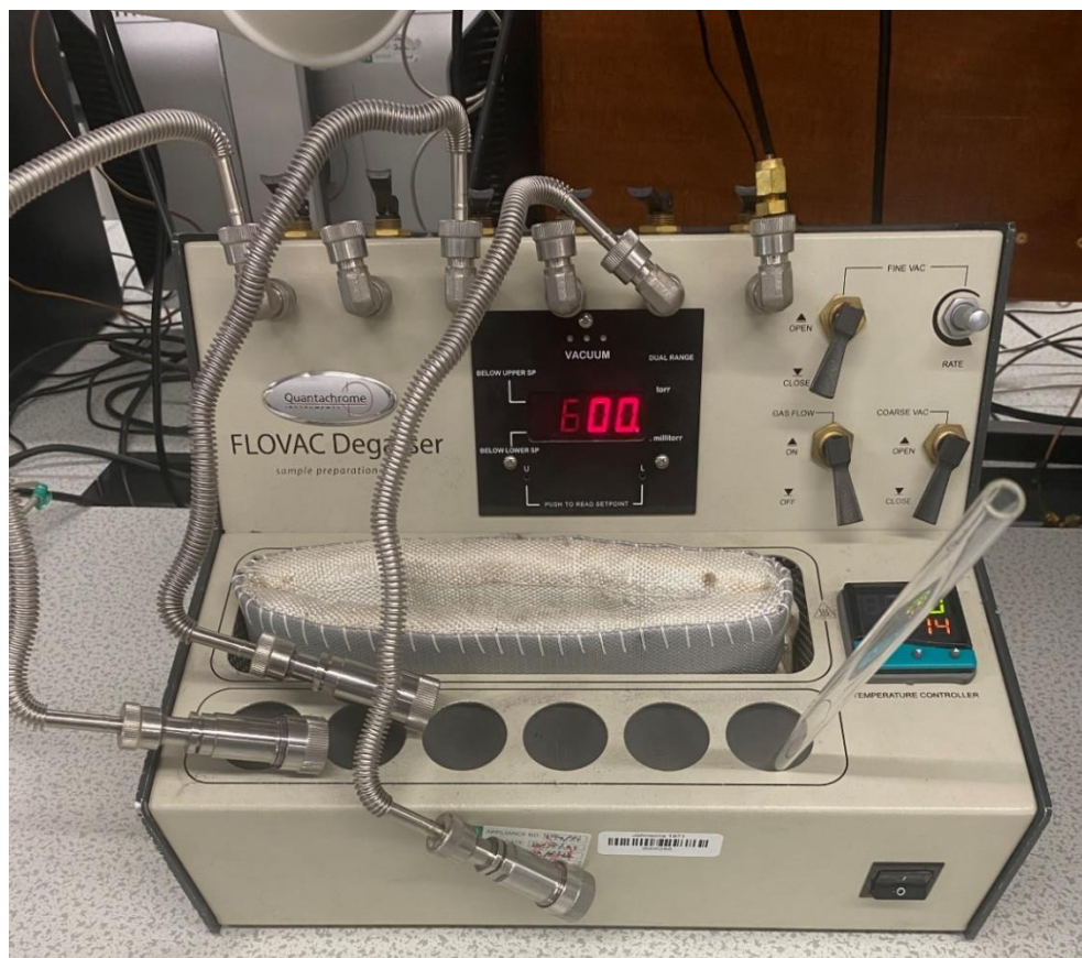
Figure 3.16: Quantachrome FloVac-Six-Port, Vacuum and flow Degasser.
