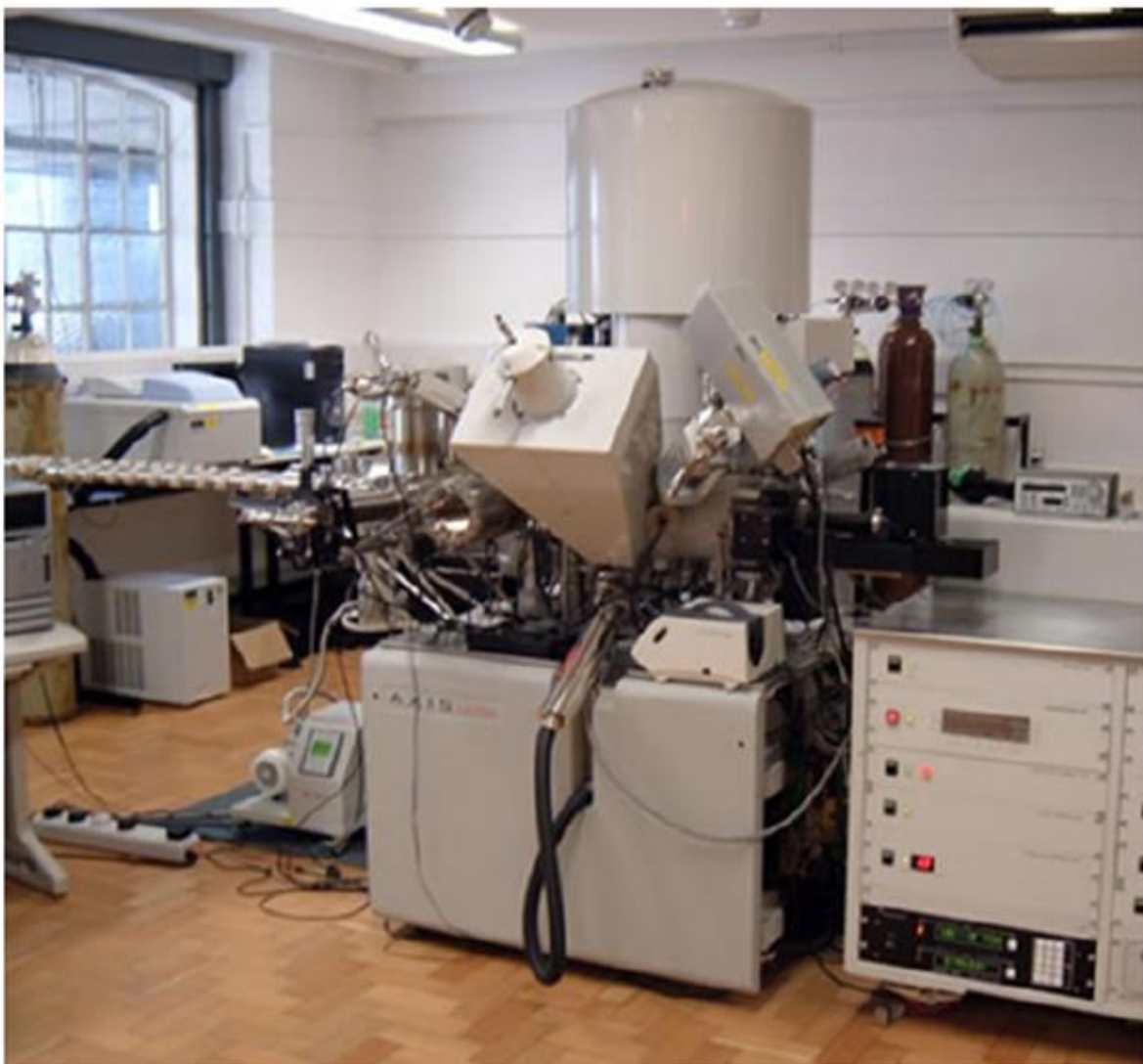
Figure 3.26: X-ray photoelectron spectroscopy (XPS), Kratos Axis Ultra DLD system.
