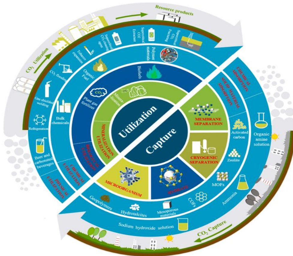
Figure 1.6: Overview diagram of CO 2 capture and utilise pathways in CCUS [22].
