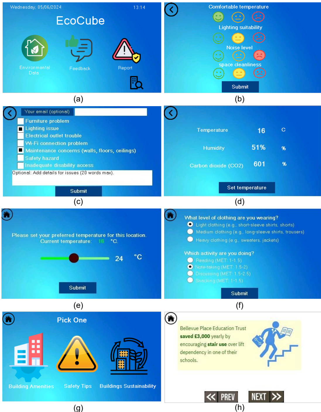
Fig. 4.10 Screenshots of the EcoCube screen: (a) main screen, (b) feedback screen, (c) reporting issue screen, (d) environmental data screen, (e) preferred temperature set by students, (f) collected data from students on thermal comfort, (g) additional building data including amenities, safety tips, and sustainability data, and (h) one of the building's sustainability information.
