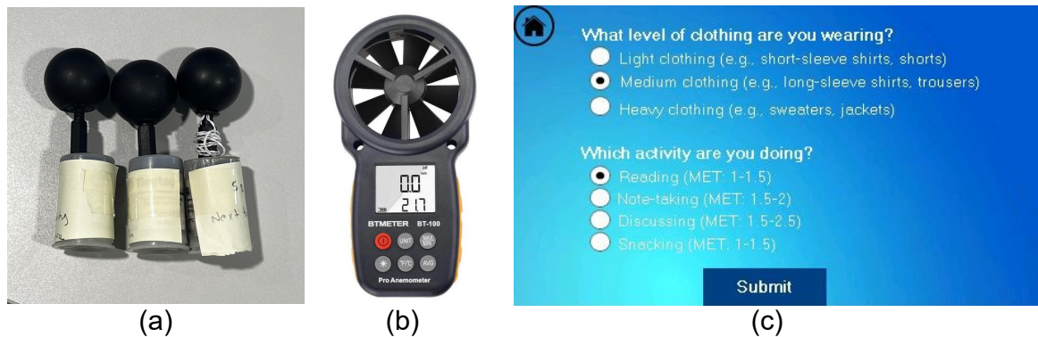
Fig. 4.11 Illustrates tools used to assess thermal comfort, including (a) wet-bulb globe temperature devices, (b) a wind speed meter, and (c) the EcoCube for gathering data on occupants' clothing levels and activity.
