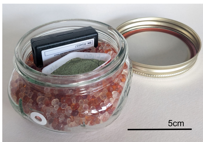
Figure 2. Vessel setup showing the placement of oxygen sensor spot, silica gel, datalogger and sample within oxygen consumption vessel.
