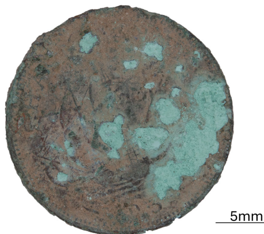
Figure 1. Copper alloy coin displaying signs of bronze disease, illustrating the physical loss of original material and heritage value that can be caused by \text{Cu}_2(\text{OH})_3\text{Cl} formation.
