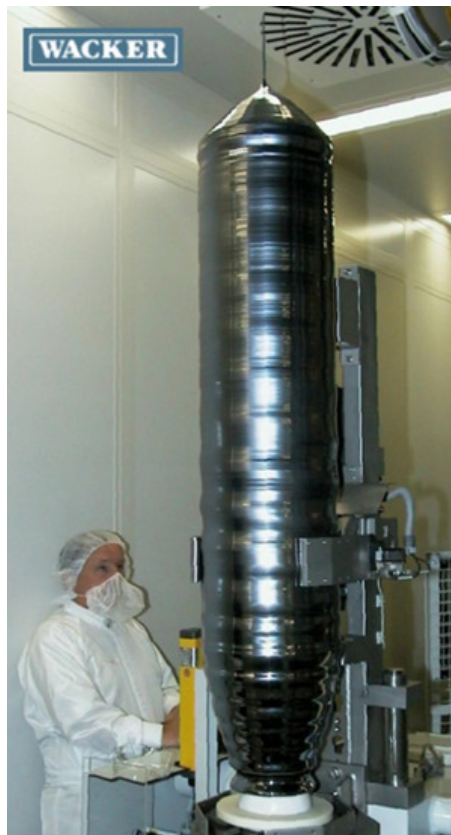
Figure 4.2: Grown silicon ingot with 300mm diameter and weighing over 250 kg. Figure taken from [85].
