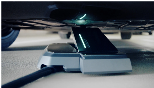
(c) VOLTERIO charging system [86]
