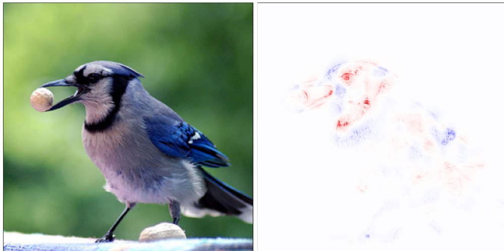
Figure 1.1: Saliency maps visually represents the contribution of input features for a task prediction by a DNN. The colour red is commonly used to represent positive contribution, and the colour blue for negative contribution. In this example input features are pixels from the image on the left, and the saliency map on the right has highlighted the pixels that contributed to the models output.
