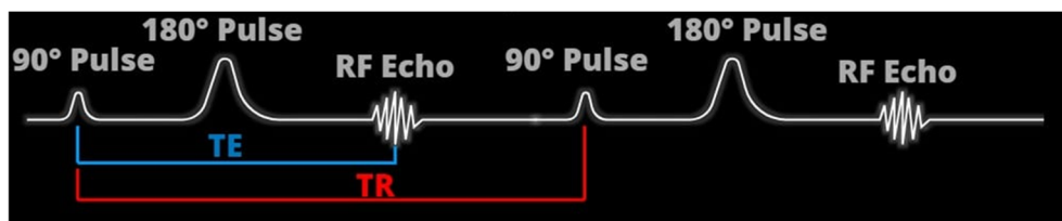
Figure 1.9 TR and TE of spin echo sequence[56].
