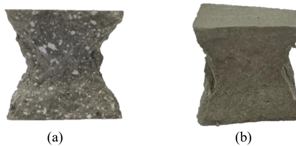
Figure 2: Photos of the cement pastes prepared with 30 wt.% replacement of cement using C in (a) dry powder form and (b) slurry form
