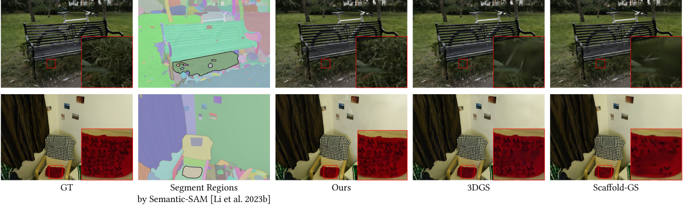
Fig. 1. 3D Gaussian Splatting (3DGS) [1] represents radiance fields through a collection of 3D primitives known as 3D Gaussians. These primitives possess radiance and opacity attributes. Despite its effectiveness, optimizing the spatial distribution of these primitives poses a challenge. In situations such as the BICYCLE scene, where the shrub grass region is not well optimized, 3DGS and other methods based on it, such as Scaffold-GS [2], struggle to accumulate sufficient gradients for split and clone operations. This limitation prohibits the achievement of detailed region reconstruction. Our proposed method utilizes segmentation information to guide spatial optimization, enabling the reconstruction of intricate regions with infrequent occurrence.
