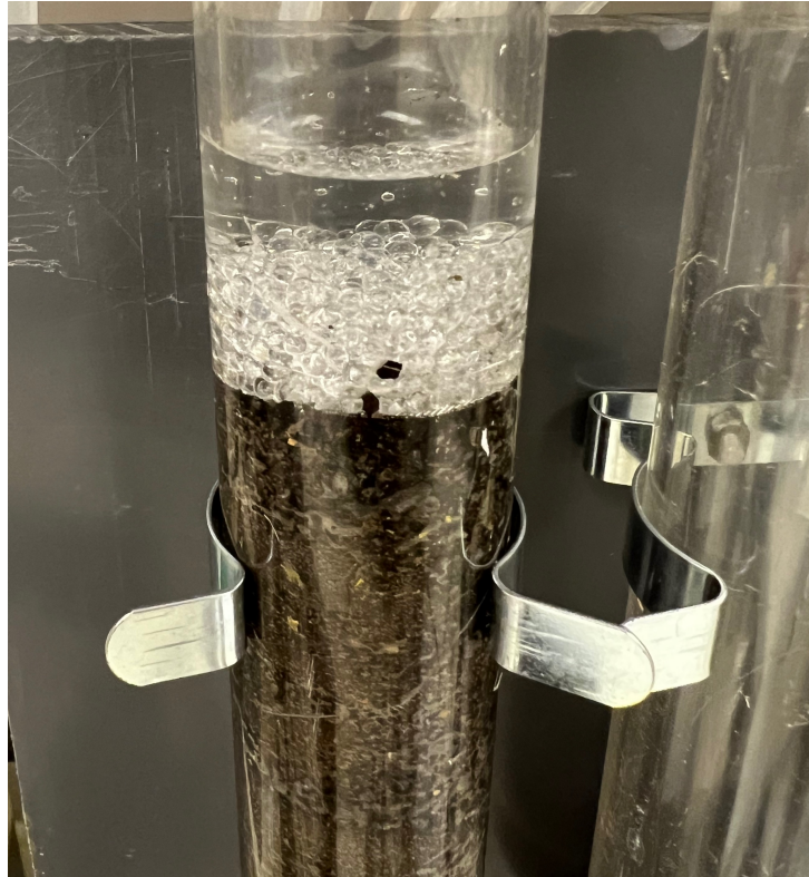
Figure 3.9 A column during test trial dosing, showing temporary ponding on the filter surface due to varying infiltration rates.
