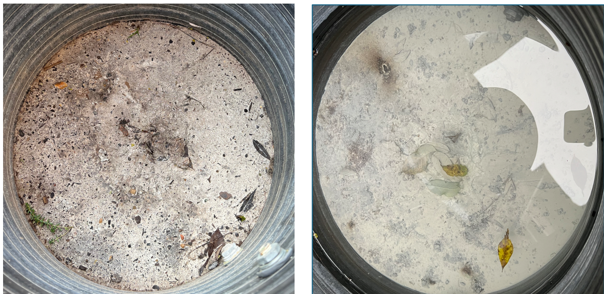
Figure 4.2 Cake layer formation decreased permeability rates and increased ponding time particularly in non-vegetated systems.
