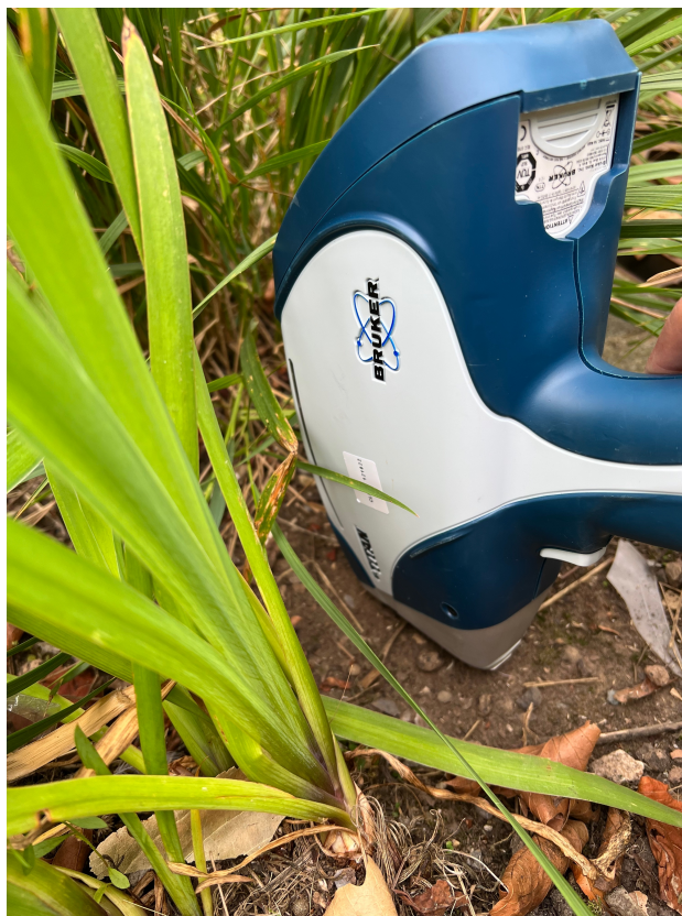
Figure 6.2 In-situ measurement of elemental composition using pXRF on a biofilter surface located on Station Terrace.
