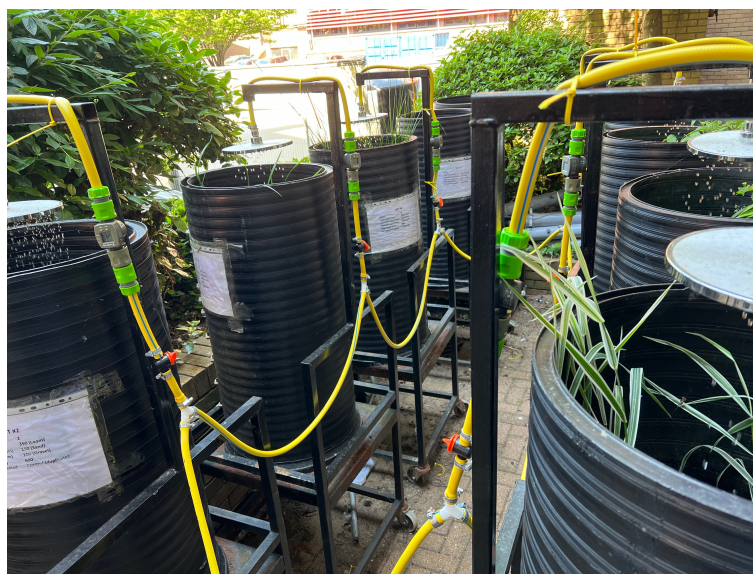
Figure 3.2 Experimental setup of large bioretention columns used to investigate the effects of vegetation on pollutant removal and system hydrology.
