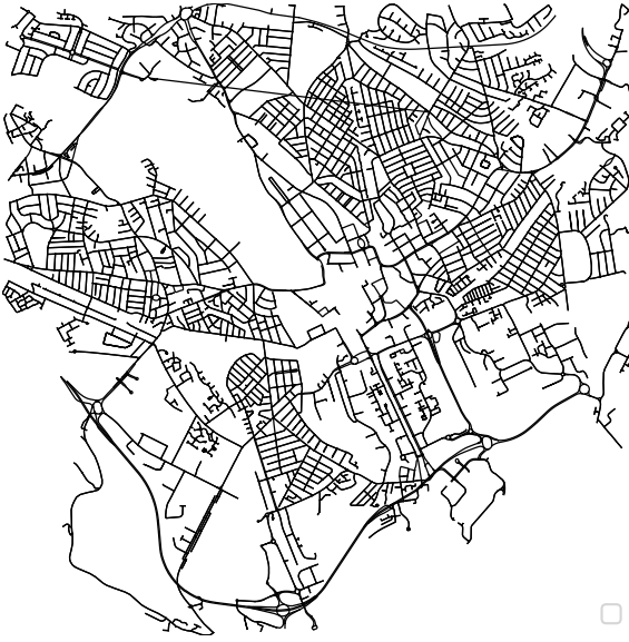
Fig. 5. Geographical street network of Cardiff city centre, extracted from OpenStreetMap (OSM) for the case study analysis. This network, covering an area within 1100 m of the city's centre, provides the underlying infrastructure for modelling EV charging station placement and user assignment within the optimisation framework.
