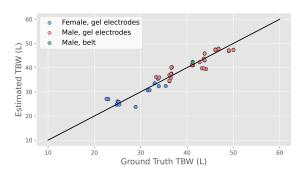
Figure 6: Predicted total body water (TBW) results compared to the ground truth TBW.
