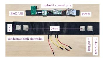
Figure 1: Trunk-facing side of measurement belt.
