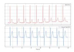
Figure 4: ECG recorded simultaneously by OxBioZ and a reference ECG device. Characteristic waves (P, QRS, T) are clearly visible in OxBioZ measurements.
