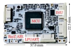
Figure 2: Custom-made OxBioZ v0.2 board combining bioimpedance analog front-end (BioZ AFE), inertial measurement unit (IMU), and microcontroller (MCU).
