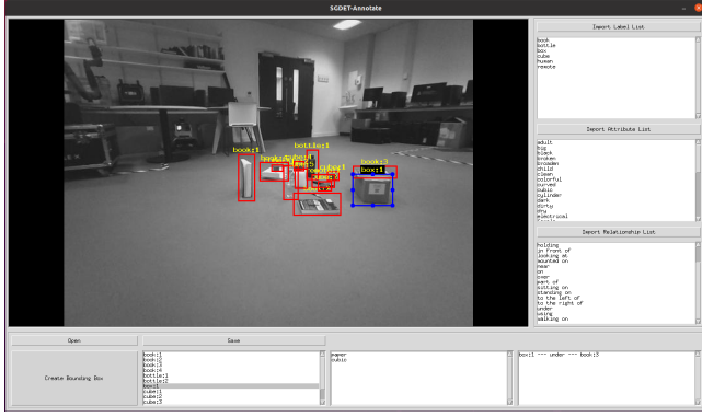
Figure 3: SGDET-Annotate (Please zoom in for the annotations): Our custom annotation tool for spatial relationship labelling. The left panel displays the robot-acquired image with editable bounding boxes; the right panel lists detected objects and available predicates. Annotators can select objects and predicates to efficiently create subject-predicate-object triplets. The tool exports annotations in both Visual Genome and YOLO formats for seamless model training and evaluation. SGDET-Annotate is open-sourced at https://github.com/harvey-ph/SGDET-Annotate .
