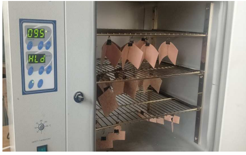
Fig. 2: View of the experimental setup used for the thermal aging
