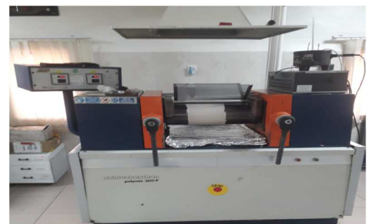
Fig. 1: The calendring machine used for the preparation of the PVC nanocomposites
