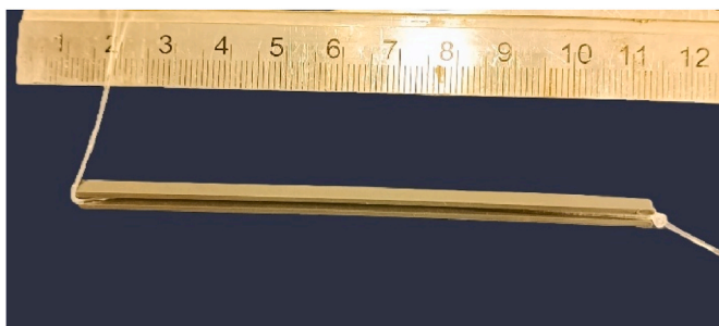
Fig. 1. Fibre knotting with U-profile to ensure effective length between the fibres of 100 mm (ruler in cm for scale).
